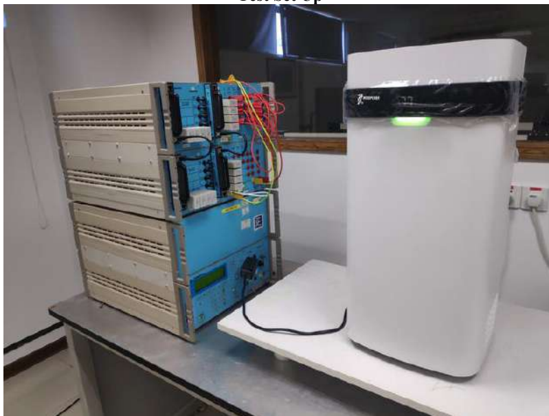
Electrical fast transient/burst & Surges & Voltage dips, short interruptions and voltage variations Test Set Up
