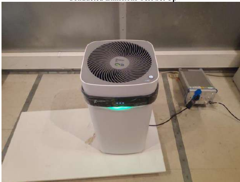
Conducted Emissions Test Set Up
