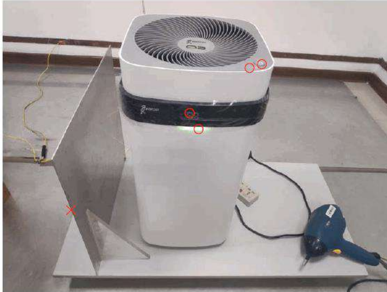
Electrostatic Discharge Test points
