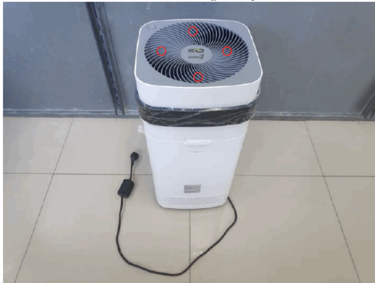
Electrostatic Discharge Test points
