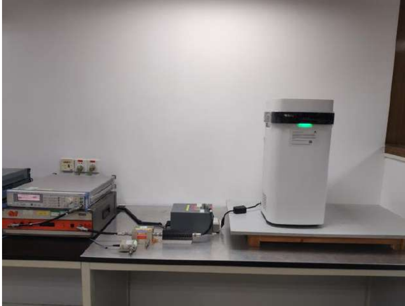
Conducted disturbances, induced by radio-frequency fields Test Set Up
