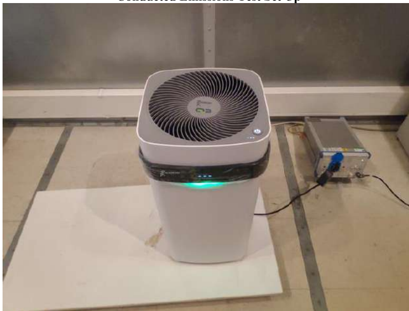
Conducted Emissions Test Set Up
