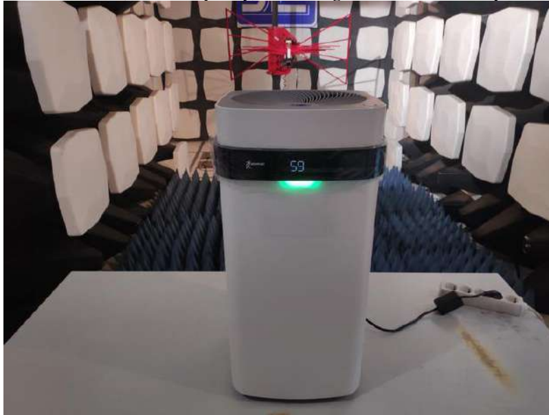
Electrical fast transient/burst & Surges & Voltage dips, short interruptions and voltage variations Test Set Up
