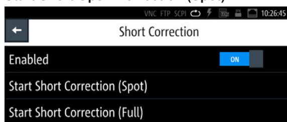
Figure 8-4: Start correction at one working point by the example of the short correction dialog
