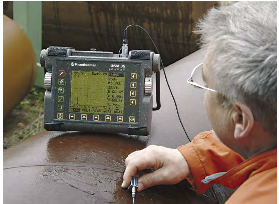
Inspection of a weld
