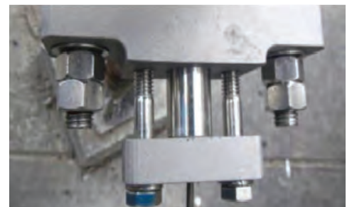
7MHz Ultra High-Temp Delay Line: transducer and mounting clamp for continuous 500°C (932°F).
