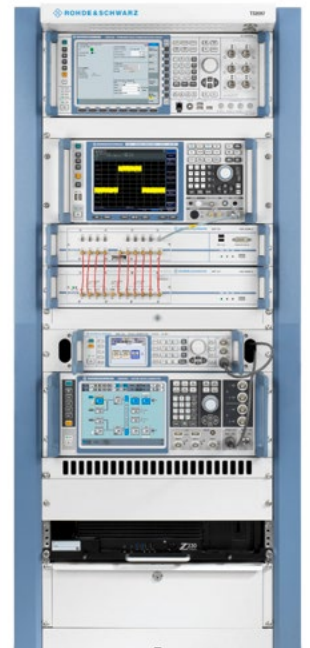
R&S®TS8997 test system with eight ports for up to eight DUTs
