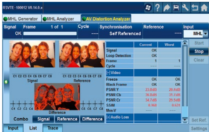
The difference picture analysis function detects video degradations and analyzes them using suitable metrics
