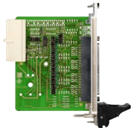
R&S®TS-PRIO4, rear I/O transmission module for R&S®TS-PIO3B, R&S®TS-PTR
