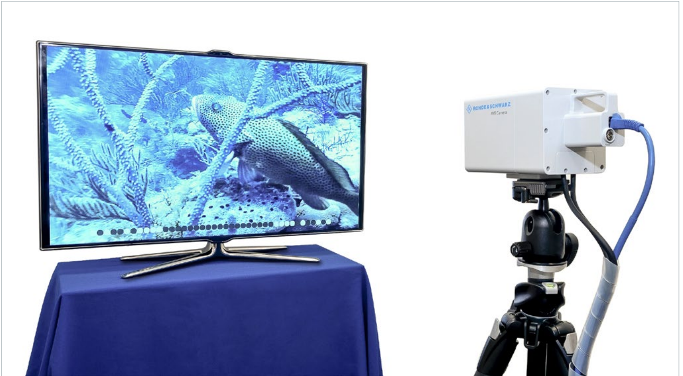
Video quality measurement directly from the TV display.
