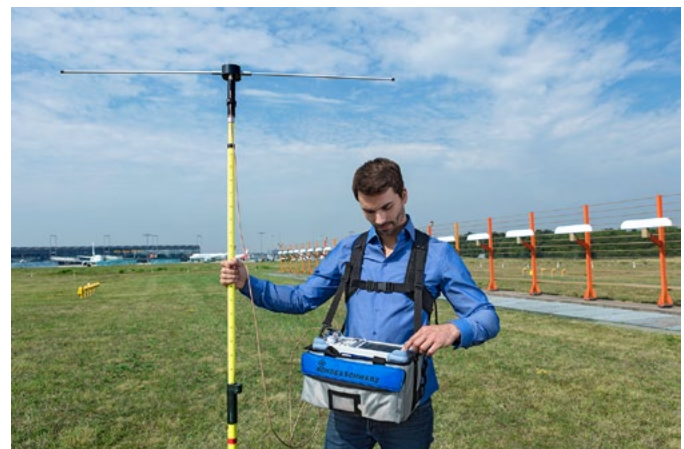
ILS measurements with R&S®EVS-Z3 ILS/VOR test antenna
