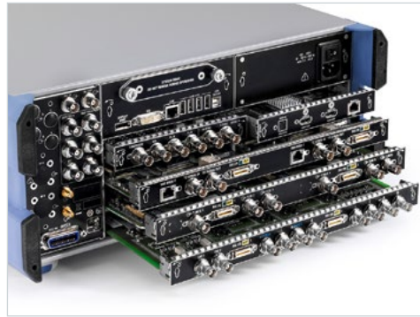
Due to its modular design, the R&S®BTC hardware can be ideally adapted to different measurement tasks
