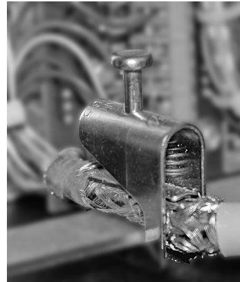
Fig. 4-27: Shield Connector Terminal With Cable
