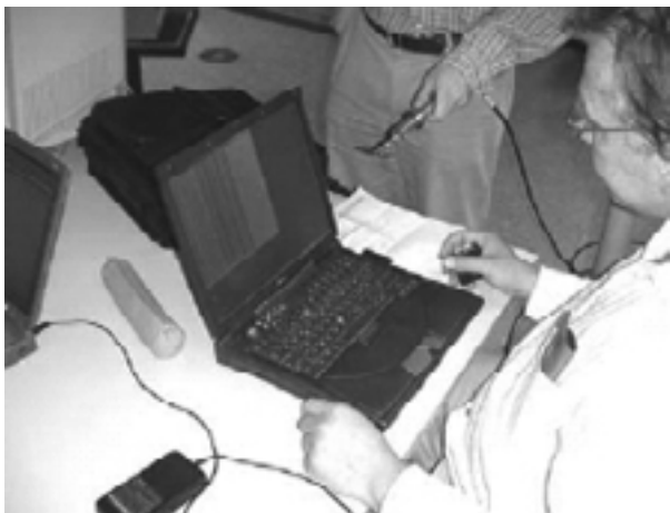
Figure 40: Scenario of a measurement at a distance of 20 cm from the notebook
