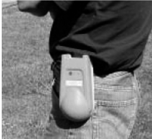
Figure 32: Example of a portable dosimeter ( Antennessa, France )
