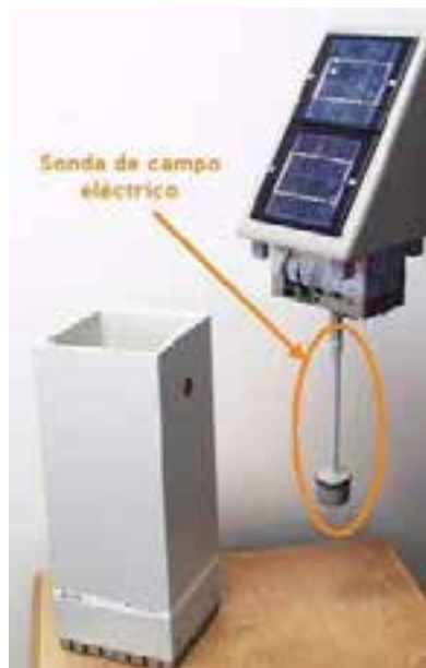
Figure A-9: Monitoring Station (MonIT, Portugal)
