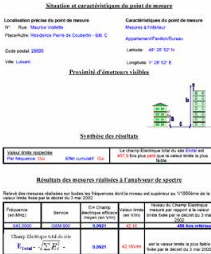
Figure A-6: Results of a spot measurement of the “Campagne de Mesures”.
