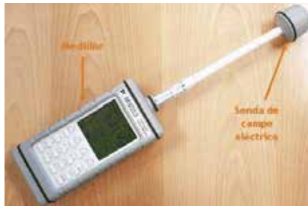
Figure 29: Portable device for broadband measurements composed of a probe and a field meter (MonIT, Portugal).
