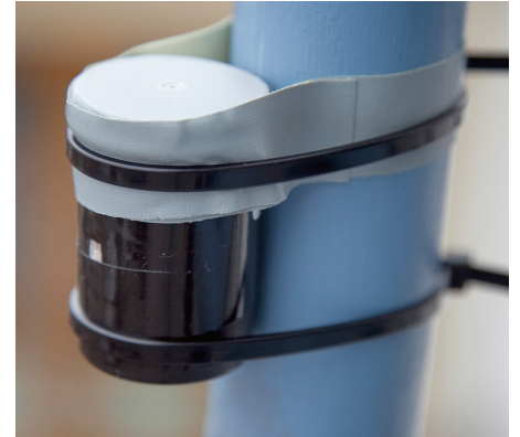
Figure 1. A mounted solargraphy can with the “shutter” open.
