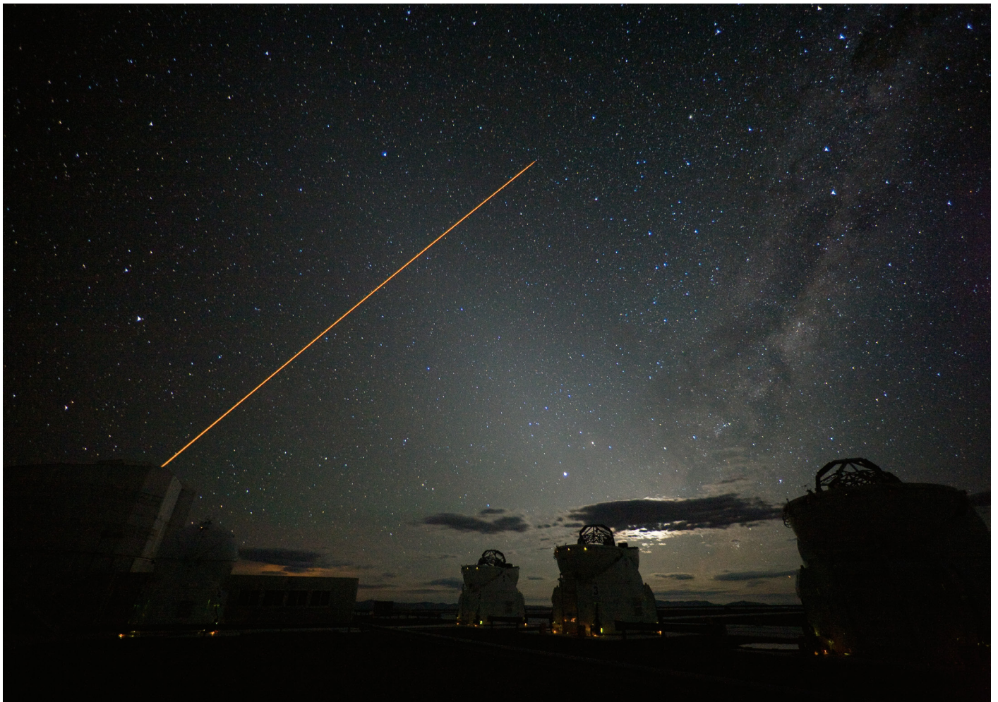
The VLT Laser Guide Star facility in action, creating a guide star for adaptive optics correction. Image taken at Paranal in 2007.
