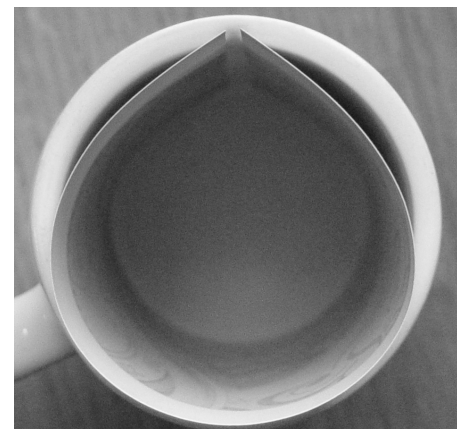
Figure 10. An illustration of how stiff paper forms itself inside a cylindrical tube. The straightening of the ends produces caustic reflections in the image.
