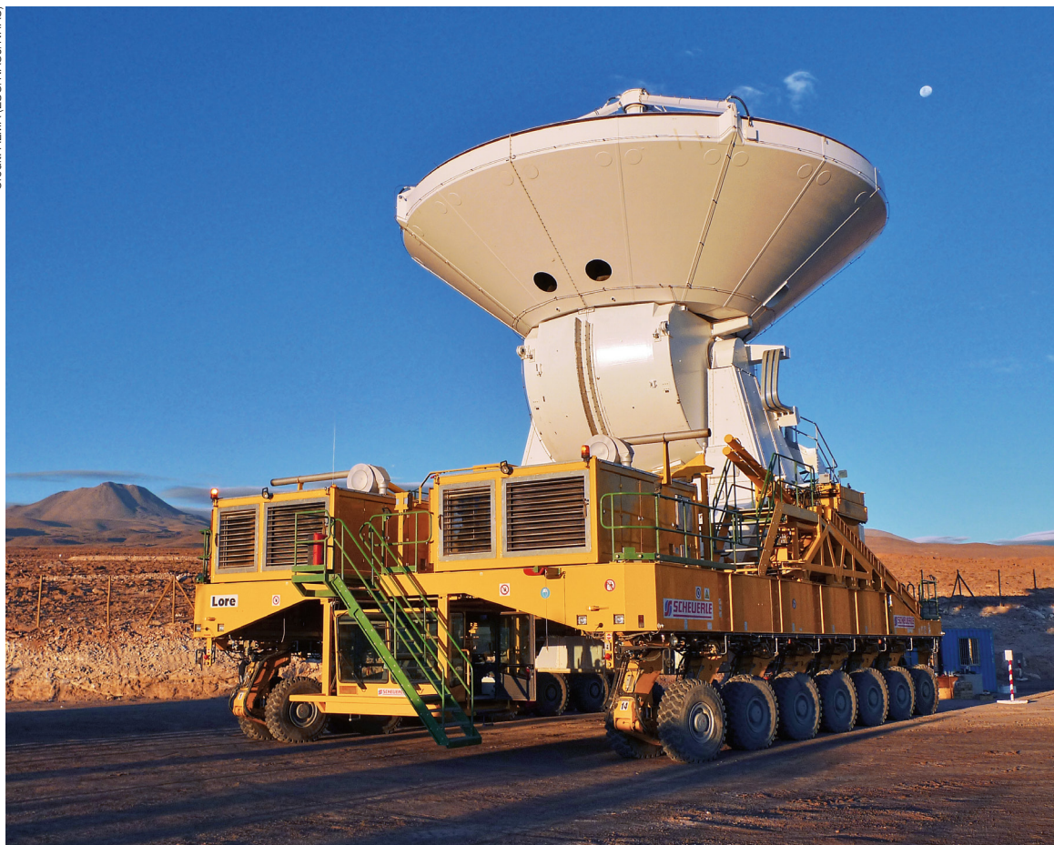
Testing of the first two fully assembled European ALMA antennas, manufactured by the AEM consortium, has recently begun at the ALMA Operations Support Facility (OSF). The image shows a European antenna being moved by one of the ALMA transporters, Lore, at the OSF.
