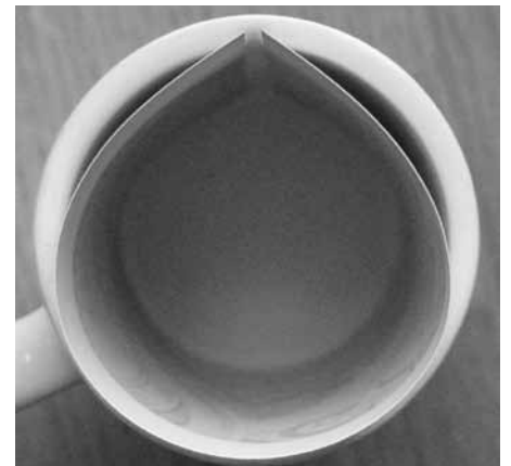
Figure 10. An illustration of how stiff paper forms itself inside a cylindrical tube. The straightening of the ends produces caustic reflections in the image.
