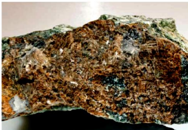
Figure 5. Dolomite cleavages from the Penn/MD Materials quarry. Field of view is 10 cm.
