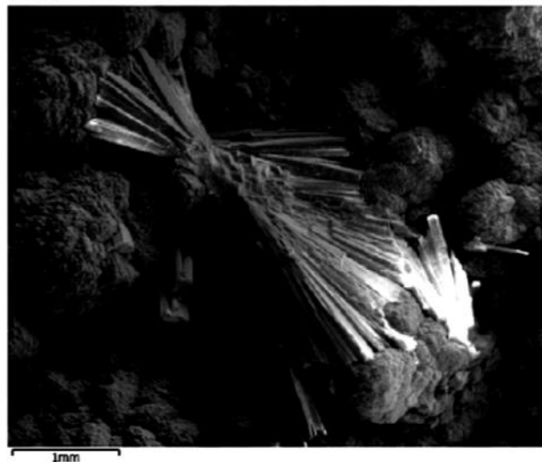
Figure 2. Scanning electron microscope image of aragonite crystals from the Penn/MD Materials quarry. Magnification is approximately 75 X.
