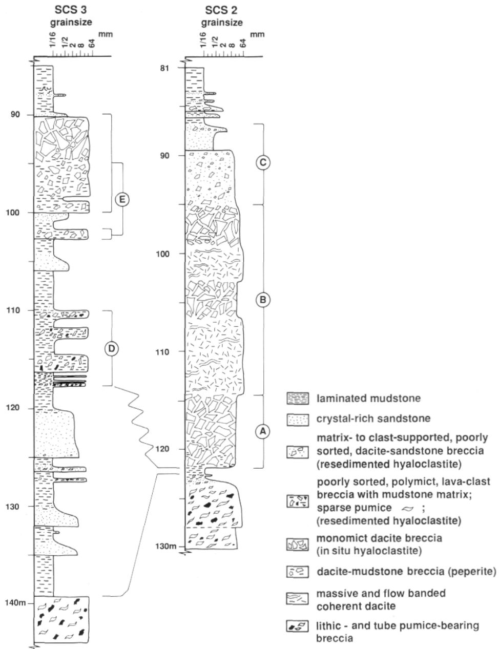
Fig. 31 Graphic lithological logs for parts of two nearby drill holes, DDH SCS2 and DDH SCS3, Sock Creek South, Mount Read Volcanics, Tasmania.
