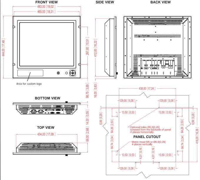
Dimensions might be shown with or without decimals and indicated as mm [inches]. Tolerance on drawings is +/- 1mm. For accurate measurements, check relevant DWG file.
