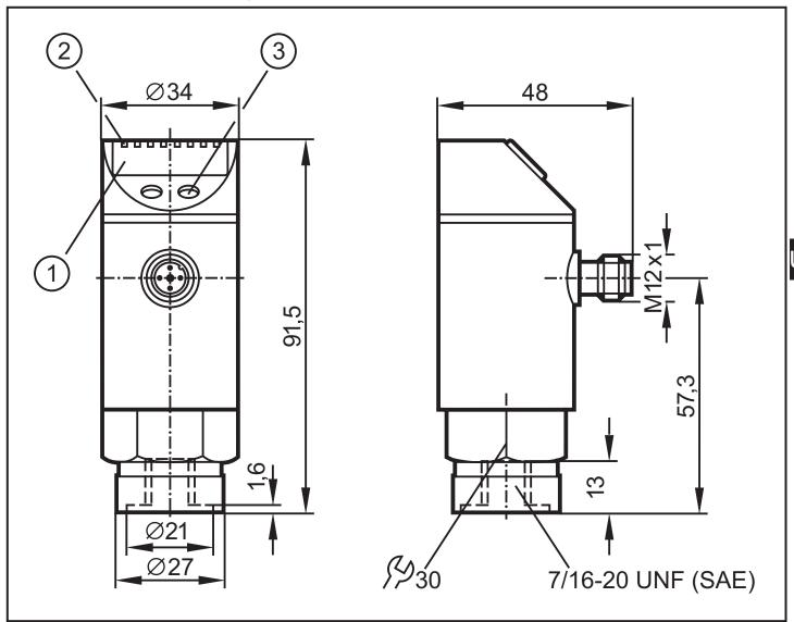
Dimensions are in millimeters
