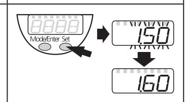
Numerical values are incremented continuously. To reduce the value: let the display move to the maximum setting value. Then the cycle starts again at the minimum setting value.
