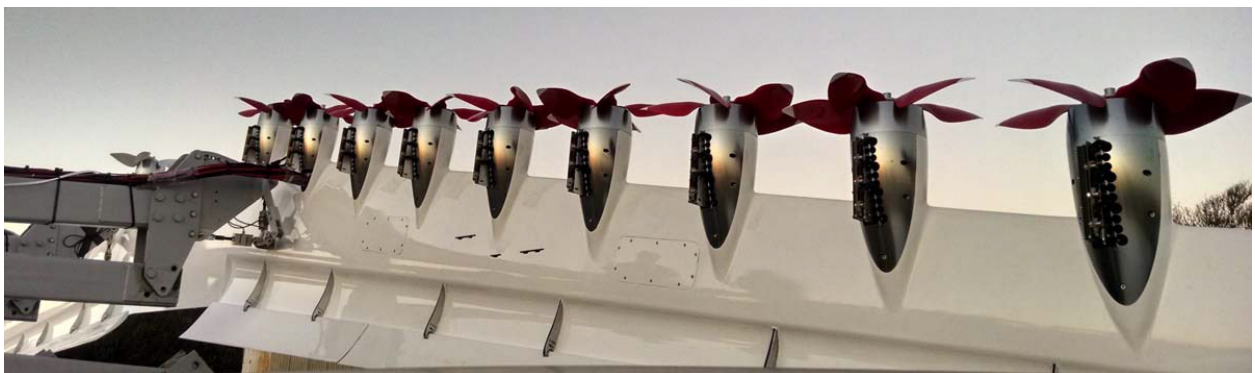
Figure 5. The underside of the HEIST wing; the flap brackets as well as the motor controllers protruding from the lower nacelle surfaces are visible. The spinners are absent. The force balance is visible at the connection between the wing and the support structure.
