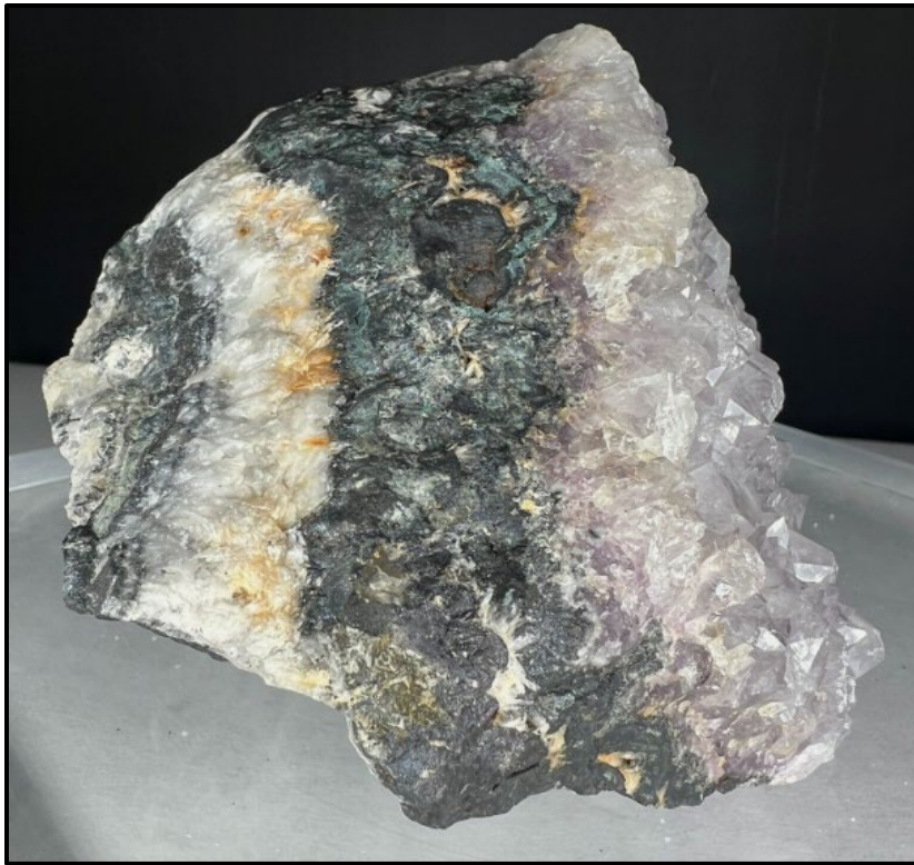
Figure 55 (left): Large specimen of stage C quartz variety amethyst crystals to about 1.5 cm deposited on banded stage B epithermal white baryte, and dark-gray sphalerite and galena ore. Specimen dimensions 18 cm x 9.5 cm x 8.5 cm. Bulldog Mountain Mine, Creede Mining District, Mineral County, Colorado. Anonymous collection. Photo credit: Phil Persson.
