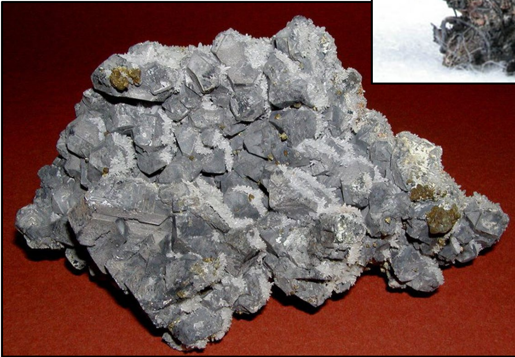
Figure 7 (above): Fine specimen of matte gray galena crystals (including a large spinel twin crystal) with chalcopyrite, quartz, and chlorite. Specimen dimensions: 15 cm x 9.0 cm x 6.5 cm. Bulldog Mountain Mine, Creede Mining District, Mineral County, Colorado. CSM Museum of Earth Sciences collection. Image credit: Mines Repository.
