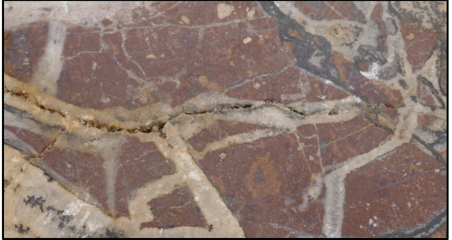
Figure 20 (above): Slice showing reddish-brown rhodochrosite with layers or inter-bands of baryte and gray sulfides. Horizontal FOV 8.0 cm. Bulldog Mountain Mine, Creede Mining District, Mineral County, Colorado. Anonymous collection. Photo credit: Author.
