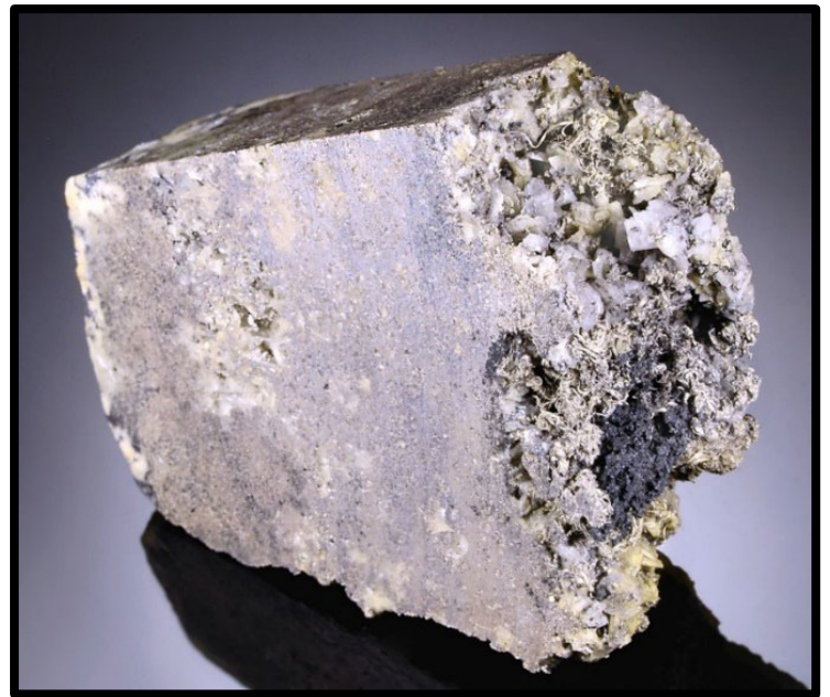
Figure 17 (above): Very thick, rich vein slice comprised mostly of wire and massive silver, acanthite (after argentite), and baryte. 67 stope, Puzzle Vein, Bulldog Mountain Mine, Creede Mining District, Mineral County, Colorado. Specimen dimensions: 7.0 cm x 5.0 cm x 2.5 cm. Anonymous collection. Photo credit: Author.
