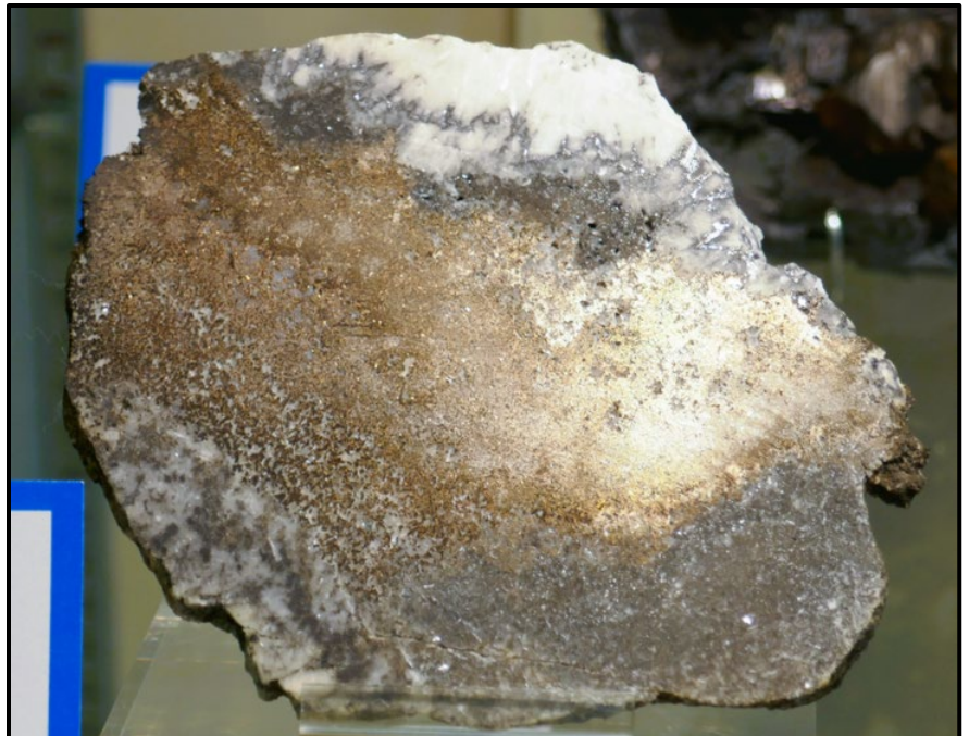
Figure 21 (right): Rich vein slice showing Stage B native silver, acanthite (paramorph after argentite), other sulfides, and baryte. From 67 Stope, Bulldog Mountain Mine, Creede Mining District, Mineral County, Colorado. CSM catalog #57643. Specimen size: 10 cm x 8.0 cm. CSM Museum of Earth Science collection. Catalog #57643. Donation from Carl Kroll collection.
