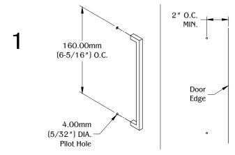
Determine the position and location for mounting on your surface. Drill your 4mm (5/32") diameter holes at 160mm (6-5/16") apart. (Note: For laminated glass door, 2" MIN. distance from the edge of the door is required.)
