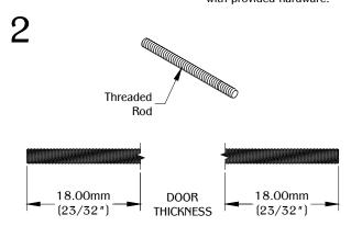
Prepare to cut the threaded rod to length by measuring your door thickness and adding 36mm (1-13/32"). Cut the rod to that exact size.
