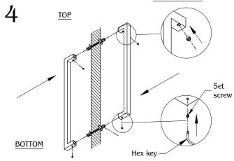
Align the door handle with the assembled base. Make sure the handle is leveled on the work surface. Use the set screw and hand-tighten the handle on both sides.
