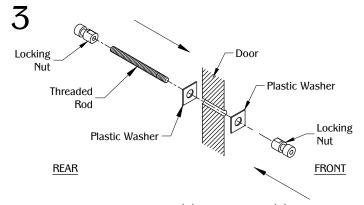
Assemble the base with (1) locking nut, (1) threaded rod, and (1) plastic washer at the back of the work surface. Align the assembly through the predrilled hole. Repeat the same assembly order from the front side. (Note: Make sure to hand tighten both sides of the assembly.)
