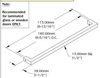
Door Thickness: 9.50mm (3/8") MIN. to 31.00mm (1-1/4") MAX.
