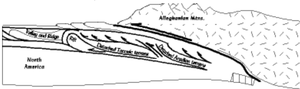
Figure 4 —The Alleghanian Orogeny, about 320–280 million years ago. As proto-Africa rides up over proto-North America, massive thrust faulting pushes the underlying bedrock westward while folding the flat sedimentary rocks beyond. Source: Fichter and Baedke (1999).
