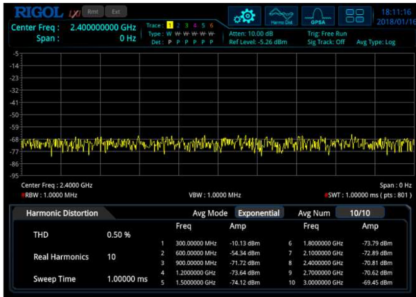
Figure 2-11 Harmonic Distortion Measurement Interface
