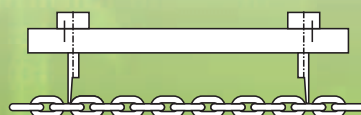
Gauge cannot be inserted: chain is to be discarded when wear >2% bzw. >3%
