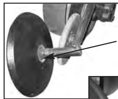
Old bearing location inside of cast wheel.
