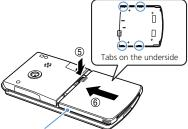
Align tabs with handset grooves and slide the cover shut.
