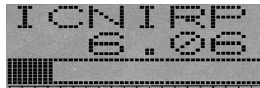
SPECTRAN® displays exposure limits both as percentage as well as a bargraph display.
