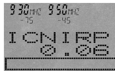
SPECTRAN® displays exposure limits both as percentage as well as a bargraph display. Our example shows approximation to the ICNIRP exposure limits by 0,06%. (Screenshot)
