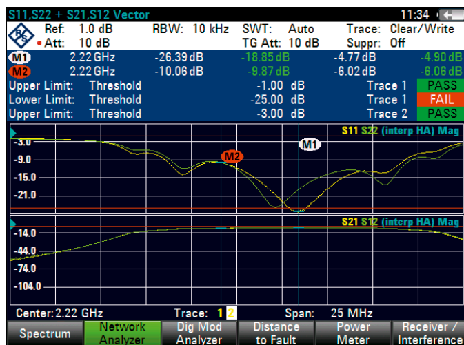
Vector network analyzer mode: For cable loss and antenna testing and characterization as well as distance to fault measurements. Two-port capability for transmission measurements
