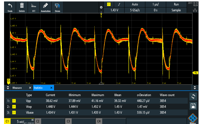
Power integrity measurement
