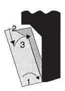
Insert the lower end of the battery (the part with the spring-blade) into the handgrip. Gently pull down against the spring so that the battery can be snapped inwards and then release the pressure.
