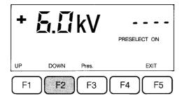
Hold F2 down until the counter content is 0000. Press F2 again to activate continuous operation. The display shows - - - -.
