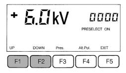
Use F1 and F2 to raise or lower the preset value. Keeping either button pressed causes the change to occur with increasing rapidity.
