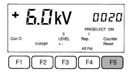
Use F5 to return to the original menu level. (This return also occurs automatically after about 10 s). The «Automatic polarity change» function is identified by «ALT. POL.» over F4 and +/- over F3.
