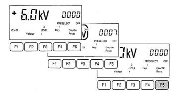
F5 sets the counter either back to 0000 or to the preset value if the preselect counter mode has been chosen.
