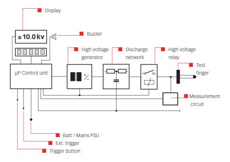
The microprocessor controls and monitors all the generator functions:
