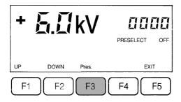
F3 switches the preselect counter operation on and off (PRESELECT ON/OFF).
