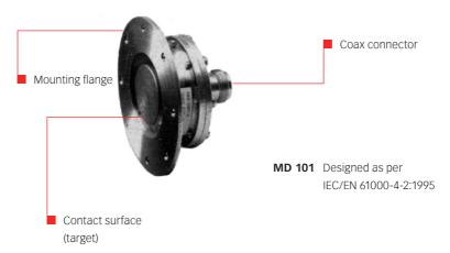
The measurement adapter type MD 101 as per informative annex B of IEC/EN 61000-4-2 serves to verify pulse amplitudes and pulse shapes. It is designed for mounting in the side wall of a Faraday cage in which an oscilloscope has been installed. This measurement adapter, also known as a «Pellegrini-Target» has the flat impedance curve to well over 1 GHz that is necessary for the purpose.
