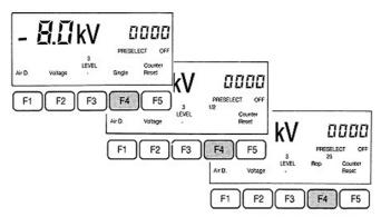
In the SINGLE mode a discharge is released each time the trigger button is pressed. The discharge is confirmed by a beep. In the REPETITIVE mode discharges are released at the chosen rate for as long as the trigger button remains pressed (no acoustic confirmation).
