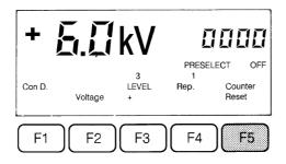
F5 first resets the counter then, when pressed a second time, branches into the preselect counter menu.
