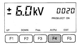
F4 switches the function «Automatic polarity change» on and off (Precondition: PRESELECT ON). The active state is shown by the polarity sign in front of the voltage alternating on the display.
