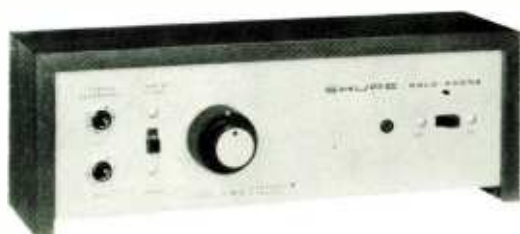
Solo/Phone amplifier by Shure drives two pairs of headsets; connects directly to program source.
