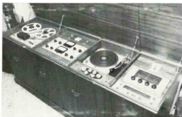
Reader Gary Gottlieb recently completed this installation. Equipment is housed in center cabinet of his own design; close-up at left shows how components are installed. Rotron fans keep units cool.
