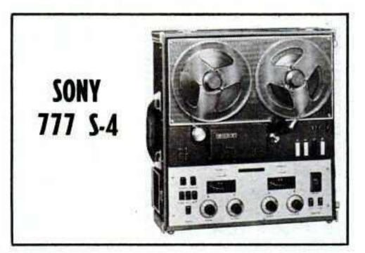
Tape speeds — 3¾ and 7½ ips. Heads — three. Motors — three. Record — 4-track mono and 4-track stereo. Playback — 2-track mono and 2 and 4-track stereo. Frequency response — 30-18,000 cps. Indicators — 2 meters. Weight — 43 lb. Other features — deck with preamps only; designed for use with SSA-777 amplifier/speaker combinations); self-contained carrying case; 2 microphone and 2 radio-phono inputs; 2 preamp and headphone outputs; monitoring; sound-on-sound; remote control. Price — less than \$695.
