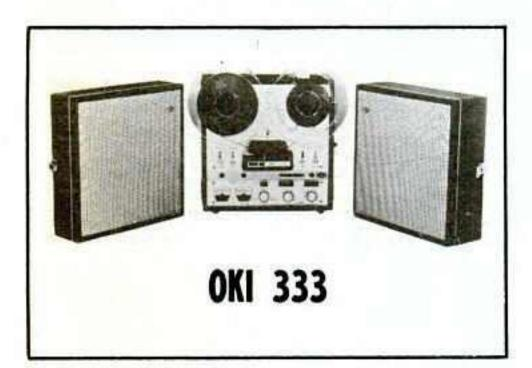
Tape speeds — 3¾ and 7½ ips. Heads — two. Motors — one. Records — 4-track mono and 4-track stereo. Playback — 4-track mono and 4-track stereo. Frequency response — 50-15,000 cps. Indicators — 2 meters. Weight — 22 lb. Other features — 2 microphone and 2 radio-phono inputs; 2 external speaker outputs; sound-on-sound; sound-with-sound; speakers built into split carrying case covers. Price — Less than \$289.95.
