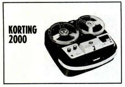
Tape speeds — 3¾ and 7 ½ ips. Heads — two. Motors — one. Record — 4-track mono. Playback — 2 and 4-track mono (4-track stereo with external preamplifier and amplifier) Frequency response — 30-20,000 cps. Indicator — electric eye. Weight — 22 lb. Other features — self-contained carrying case; microphone and radio-phono inputs; 2 stereo head outputs; 2 preamp and external speaker outputs; built-in speaker. Price — \$199.95.
