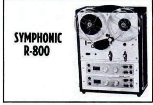
Tape speeds — 1%, 3% and 7½ ips. Heads — two. Motors — one. Record — 4-track mono and 4-track stereo. Playback — 4-track mono and 4-track stereo. Frequency response — 50-15,000 cps. Indicators — 2 meters. Weight — 35 lb. Other features — self-contained carrying case; 2 microphone and 2 radio-phono inputs; 2 preamp, 2 external speaker headphone outputs; automatic shutoff; electric braking; all transistor. Price — \$249.95.
