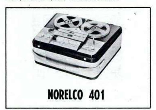
Tape speeds — 15/16,  $1\frac{7}{8}$ ,  $3\frac{3}{4}$  and  $7\frac{1}{2}$  ips. Heads — two. Motors — one. Record — 4track mono and 4-track stereo. Playback -4-track mono and 4-track stereo. Frequency response — 50-18,000 cps. Indicator— neon light. Weight — 39 lb. Other features — selfcontained carrying case; microphone, 2 radiophono inputs; 1 preamplifier, 2 external speaker outputs; sound-on-sound; automatic shutoff; monitoring; 1 speaker in recorder and 1 in carrying case cover.
