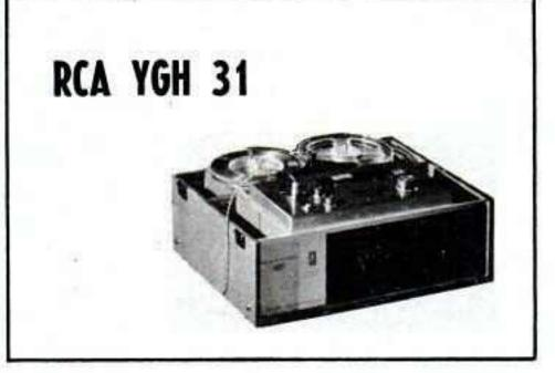
Tape speeds — 1%, 3% and 7½ ips. Heads — two. Motors — one. Record — 4-track mono. Playback — 4-track mono. Frequency response — 50-15,000. Indicator — meter. Weight — not available. Other features — self-contained carrying case; microphone and radio-phono inputs; preamp output; built-in speaker. Price — \$129.95.
