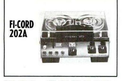
Tape speeds — 3¾ and 7½ ips. Heads — two. Motors — one. Record — 2-track mono. Playback — 2-track mono. Frequency response — 50-12,000 cps. Indicator — meter. Weight — 6¾ lb. Other features — powered by 7 1.4-volt mercury batteries, or AC or car battery with accessory adapters; microphone input; preamplifier and external speaker outputs; remote control; built-in speaker. Price — \$350.
