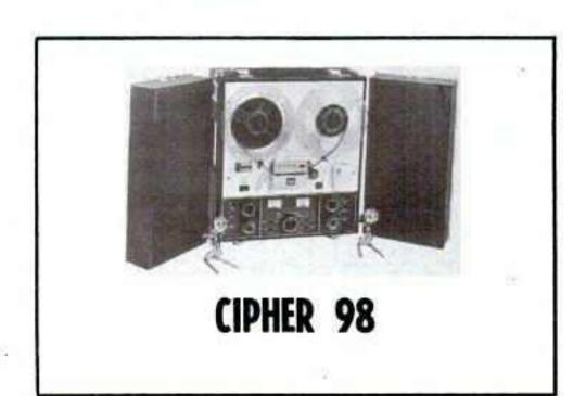
Tape speeds —  $1\frac{7}{8}$ ,  $3\frac{3}{4}$  and  $7\frac{1}{2}$  ips. Heads three. Motors — one. Record — 4-track mono and 4-track stereo. Playback — 4-track mono and 4-track stereo. Frequency response — 35-
