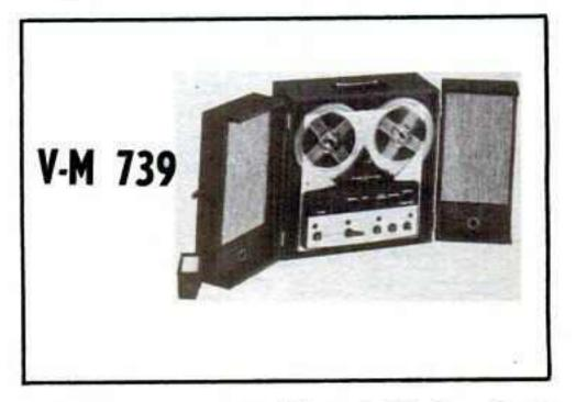
Tape speeds — 1%, 3% and 7½ ips. Heads — one. Motors — one. Record — 4-track mono and 4-track stereo. Playback — 4-track mono and 4-track stereo. Frequency response — 50-15,000 cps. Indicators — 2 neon lights. Weight — 28 lb. Other features — self-contained carrying case; 2 microphone inputs; 2 preamp and 2 external speaker outputs; slide projector sync provision; sound-with-sound; 2 speakers built into split carrying case cover. Price — \$209.95.
