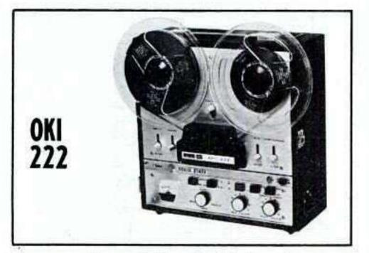
Tape speeds — 33/4 and 71/2 ips. Heads two. Motors — one. Record — 4-track mono. Playback — 4-track mono and 4-track stereo (with external preamplifier and amplifier). Frequency response — 50-15,000 cps. Indicator - meter. Weight - 151/2 lb. Other features self-contained carrying case; microphone and radio-phono inputs; phono and radio-phono inputs; preamplifier and tape head outputs; soundon-sound; sound-with-sound; built-in speaker. Price — \$179.95.
