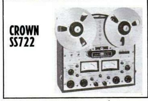
Tape speeds — 1%, 3% and 7½ ips. Heads — two. Motors — three. Record — 2-track mono and 2-track stereo. Playback — 2-track mono and 2-track stereo. Frequency response — 50-25,000 cps. Indicators — 2 meters. Weight — 50 lb. Other features — deck, with preamps only; 2 microphone and 2 radio-phono inputs; 2 preamp, and mono and stereo headphone outputs; automatic stop. 4-track model also available. Price — \$995.
