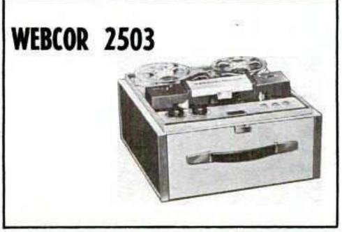
Tape speeds —  $1\frac{7}{8}$ ,  $3\frac{3}{4}$  and  $7\frac{1}{2}$  ips. Heads — two. Motors — one. Record — 4-track mono. Playback — 4-track mono. Frequency response — 100-15,000 cps. Indicator — meter. Weight — 21 lb. Other features — self-contained carrying case; microphone and radiophono inputs; preamp and external speaker outputs; 2 built-in speakers. Price - \$159.95.
