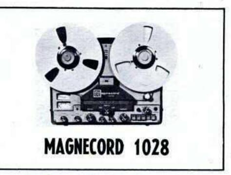
Tape speeds —  $7\frac{1}{2}$  and 15 ips. Heads three. Motors — three. Record — 2-track mono and 2-track stereo. Playback - 2-track mono and 2-track stereo. Frequency response — 35-18,000 cps. Indicators — 2 meters. Weight — 47 lb. Other features — deck, with preamps and 2 monitoring amplifiers; 2 microphone, 2 radio-phono and 2 auxiliary inputs; preamp outputs. Price — \$995.
