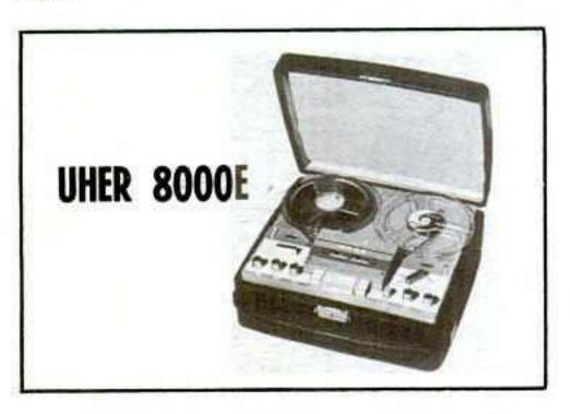
Tape speeds — 15/16, 1%, 3% and 7½ ips. Heads — four. Motors — one. Record — 4-track mono and 4-track stereo. Playback — 4-track mono and 4-track stereo. Frequency response — 50-20,000 cps. Indicators — 2 meters. Weight — 19 lb. Other features — self-contained carrying case; microphone, radio and phono inputs; 2 remote control; external speakers, headphone outputs; sound-on-sound; sound-with-sound; echo effects; slide projector sync; monitoring; 2 built-in speakers. Price — \$419.95.
