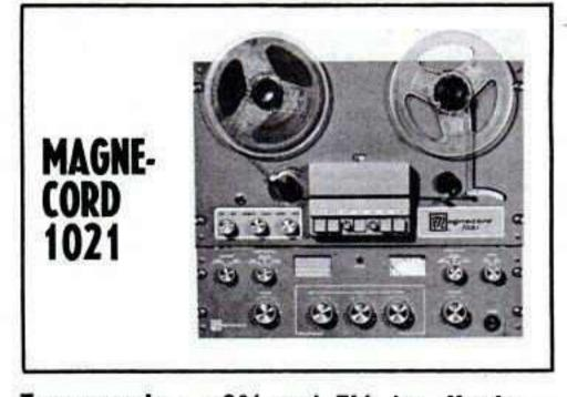
Tape speeds — 3¾ and 7½ ips. Heads — three. Record — full track mono. Playback — full and 2-track mono. Frequency response — 45-18,000 cps. Indicator — meter. Weight — 47 lb. Other features — deck, with preamp and monitoring amp; 3 microphone and 1 radio-phono input; preamp, speaker, headphone and sound-on-sound; monitoring speaker. Price — \$708.
