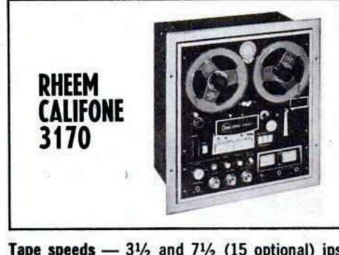
Tape speeds — 3½ and 7½ (15 optional) ips. Heads — three. Motors — three. Record — 4-track mono and 4-track stereo. Playback — 4-track mono and 4-track stereo. Frequency response — 40-18,000 cps. Indicators — 2 meters. Weight — 54 lb. Other features — deck, with preamps only. 2 microphone and 2 radio-phono inputs; 2 preamp, headphone outputs. Automatic shutoff; sound-on-sound; sound-
