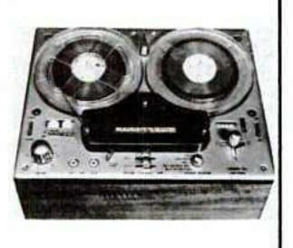
Tape speeds —  $1\frac{7}{8}$ ,  $3\frac{3}{4}$  and  $7\frac{1}{2}$  ips. Heads — two. Motors — one. Record — 4-track mono and 4-track stereo. Playback - 4-track mono and 4-track stereo. Frequency response 40-16,000 cps. Indicators — electric eye. Weight — 27 lb. Other features — wood base, 2 microphone and 2 radio-phono inputs; 2 preamp and 2 external speaker outputs; soundon-sound; monitor; 2 built-in speaker. Price **— \$449.50.**
