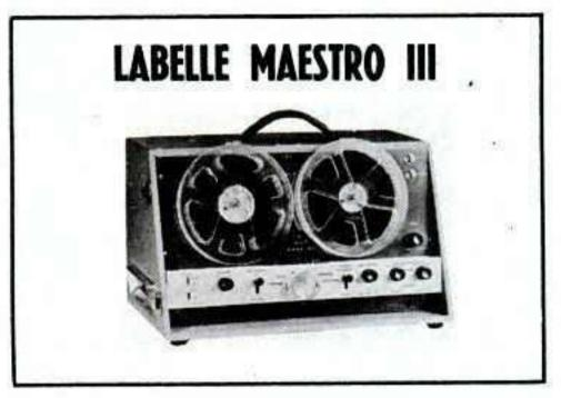
Tape speeds — 3¾ and 7½ ips. Heads — one. Motors — one. Record — 2-track mono. Playback — 2-track mono. Frequency response — 50-15,000 cps. Indicator — 2 neon lamps. Weight — 28 lb. Other features — self-contained carrying case; microphone and radio-phono inputs; external speaker output; slide projector sync pulse; speaker built into carrying case cover. Price — \$375.
