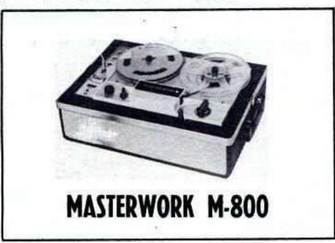
Tape speeds —  $1\frac{7}{8}$ ,  $3\frac{3}{4}$  and  $7\frac{1}{2}$  ips. Heads — two. Motors — one. Record — 2-track mono. Playback — 2-track mono. Frequency response —100-10,000 cps. Meter — Indicator — meter. Weight — 25 lb. Other features — self-contained carrying case; microphone and radiophono inputs; external speaker and earphone outputs; monitoring; built-in speaker. Price -\$99.95.
