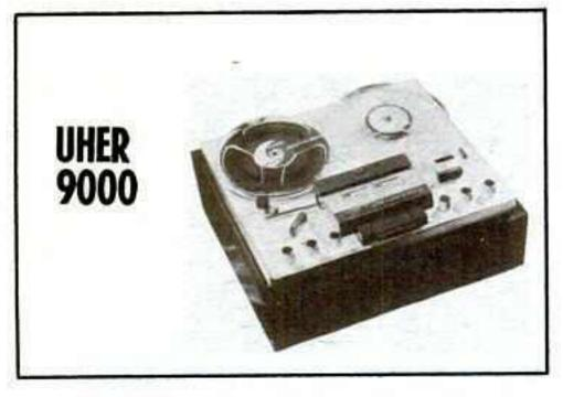
Tape speeds — 3¾ and 7½ ips. Heads — three. Motors — one. Record — 4-track mono and 4-track stereo. Playback — 4-track mono and 4-track stereo. Frequency response — 20-20,000 cps. Indicators — 2 meters. Weight — 22 lb. Other features — deck, with preamps only: metal or wood base; 2 microphone (low impedance), 2 radio, and 2 phono inputs; 2 preamp and headphone outputs; voice actuated recording; slide sync provision; automatic shutoff. Price — not available.
