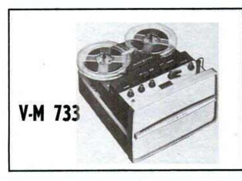
Tape speeds — 1%, 3% and 7½ ips. Heads — one. Motors — one. Record — 4-track mono. Playback — 4-track mono. Frequency response — 50-15,000 cps. Indicator — electric eye. Weight — 22 lb. Other features — self-contained carrying case; microphone input; preamp, external speaker, and headphone output; slide projector sync provision; built-in speaker. Price — \$169.95.
