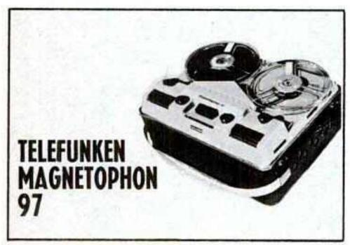
Tape speeds —  $1\frac{7}{8}$ ,  $3\frac{3}{4}$  nd  $7\frac{1}{2}$  ips. Heads — two. Motors — one. Record — 4-track mono and 4-track stereo. Playback — 4-track mono and 4-track stereo. Frequency response — 30-18,000 cps. Indicator — electric eye. Weight — 29 lb. Other features — self-contained carrying case; 2 microphone and 4 radiophono inputs; 2 preamp, 2 external speaker and 2 headphone outputs; sound-on-sound; sound-with-sound; one speaker built-in, one in
