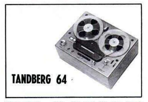
Tape speeds — 1%, 3% and 7½ ips. Heads — three. Motors — one. Record — 4-track mono and 4-track stereo. Playback — 4-track mono and 4-track stereo. Frequency response — 40-16,000 cps. Indicators — 2 electric eyes. Weight — 25 lb. Other features — wood base; deck with preamps only; 2 microphone, 2 radio-phono and 2 auxiliary inputs; 2 preamp outputs; sound-on-sound echo, sound-with-sound. Price — \$498.
