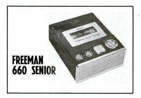
Tape speeds — 1% (with special capstan sleeve) 3% and 7½ ips. Heads — two. Motors — one. Record — 2-track mono. Playback — 2-track mono. Frequency response — 65-15,000 cps. Indicator — meter. Weight — 8½ lb. Other features — powered by 6 penlight batteries or AC with built-in adapter; remote control microphone and radio-phono inputs; earphone and external speaker outputs; stroboscope control 3% and 7½ ips; and built-in speaker. Price — \$199.50.
