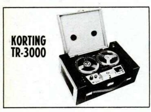
Tape speeds — 3¾ and 7½ ips. Heads — two. Motors — one. Record — 4-track mono and 4-track stereo. Playback — 2 and 4-track mono and 4-track stereo. Frequency response — 30-20,000 cps. Indicator — electric eye. Weight — 30 lb. Other features — self-contained carrying case; 2 microphone, 2 radio-phono, and 2 auxiliary inputs; 2 tape head, 2 preamp, 2 external speaker, and headphone outputs; monitor; sound-on-sound; provision for slide projector sync; 2 built-in speakers. Price — \$299.95.
