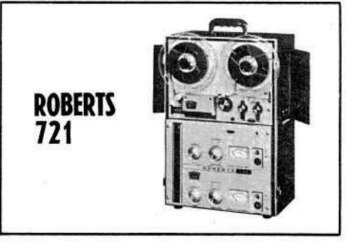
Tape speeds — 3¾ and 7½ (15 optional) ips. Heads — two. Motors — one. Record — 4-track mono and 4-track stereo. Playback — 4-track mono and 4-track stereo. Frequency response — 40-17,000 cps. Indicators — 2 meters. Weight — 49 lb. Other features — self-contained carrying case; 2 microphone and 2 radio-phono inputs; 2 preamp, 4 headphone, 2 extension speaker, 2 sound head outputs; sound-with-sound; sound-on-sound; monitoring; automatic shutoff. Price — \$359.95.
