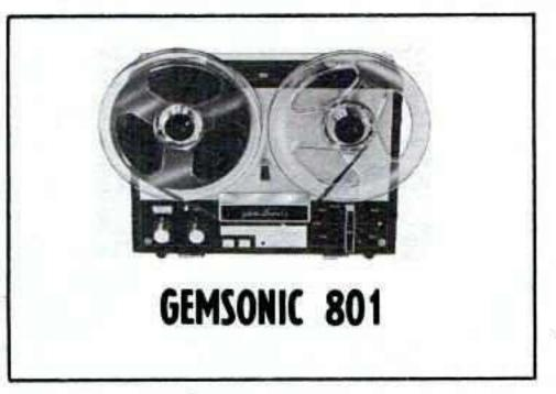
Tape speeds — 3¾ and 7½ ips. Heads — two. Motors — one. Racord — 4-track mono. Playback — 4-track mono and 4-track stereo (with external amp and speaker). Frequency response — 50-12,000 cps. Indicator — meter. Weight — 13 lb. Other features — self-contained carrying case; microphone and radio-phono inputs; extension speaker; preamp and sound head outputs; automatic shutoff. Price — \$99.95.
