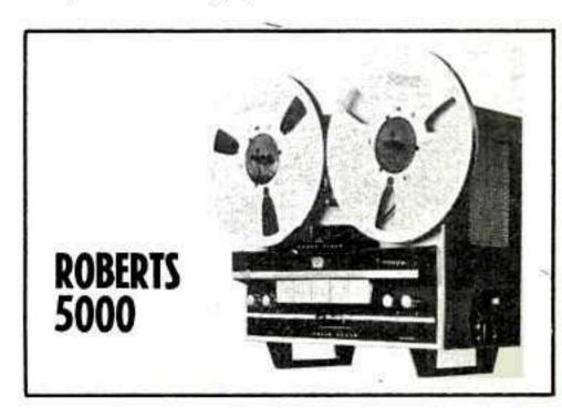
Tape speeds — 3¾ and 7½ (15 optional) ips. Heads — three. Motors — three. Record — 4-track mono and 4-track stereo. Playback — full, 2- and 4-track mono and 2- and 4-track stereo. Frequency response — 30-22,000 cps. Indicators — 2 meters. Weight — not available. Other features — 2 microphone and 2 radio-phono inputs; 2 preamp, 2 external speaker, headphone outputs; cross field head; sound-on-sound; all transistor; 2 built-in speakers. Price — \$699.95.
