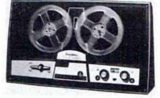
Tape speeds — 15/16, 1%, 3% and 7½ ips. Heads — two. Motors — one. Record — 4-track mono and 4-track stereo. Playback — 4-track mono and 4-track stereo. Frequency response — 50-18,000 cps. Indicator — meter. Weight — 26 lb. Other features — self-contained carrying case; 2 microphone and 2 radio-phono inputs; 2' preamp and 2 external speaker outputs; sound-on-sound, sound-with-sound; automatic shutoff; 2 built-in speakers. Price — \$179.95.
