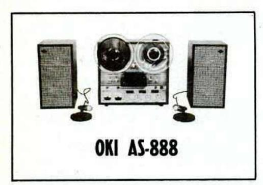
Tape speeds — 3¾ and 7½ ips. Heads — three. Motor — one. Record — 4-track mono and 4-track stereo. Playback — 4-track mono and 4-track stereo. Frequency response — 40-18,000 cps. Indicators — 2 meters. Weight — not available. Other feaures — walnut base; 2 microphone, 2 radio-phono, and 2 auxiliary inputs; 2 preamp and 2 speaker outputs; sound-on-sound; sound-with-sound; 2 bookshelf speakers in walnut enclosures. Price — \$489.85.
