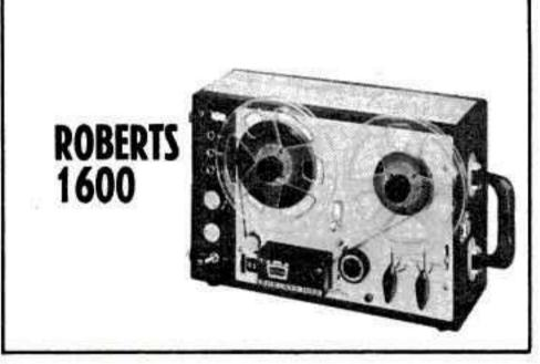
Tape speeds — 1%, 3% and 7½ ips. Heads two. Motors — one. Record — 2-track mono. Playback — 2-track mono. Frequency response —50-15,000 cps. Indicator — meter. Weight —22 lb. Other features — microphone and radio-phono inputs; external speaker output; built-in speaker. Price — \$169.95.
