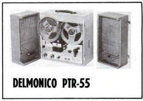
Tape speeds — 3¾ and 7½ ips. Heads — two. Motors — one. Record — 4-track mono and 4-track record. Playback — 4-track mono and 4-track mono and 4-track mono and 4-track stereo. Frequency response — 50-12,000 cps. Indicators — 2 meters. Weight — 55 lb. Other features — self-contained carrying cases; 2 microphone and 2 radio-phono inputs; 2 preamp and 2 extension speaker outputs; 2 built-in speakers. Price — \$169.95.
