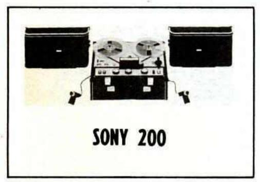
Tape speeds — 3¾ and 7½ ips. Heads — two. Motors — one. Record — 4-track mono and 4-track stereo. Playback — 4-track mono and 4-track stereo. Frequency response — 50-14,000 cps. Indicators — 2 meters. Weight — 27 lb. Other features — self-contained carrying case; 2 microphone and 2 radio-phono inputs; 2 preamp and 2 external speaker outputs; sound-on-sound; 2 speakers in split carrying case cover. Price — less than \$199.50.
