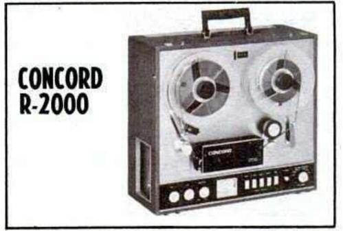
Tape speeds — 3¾ and 7½ ips. Heads — four. Motors — three. Record — 4-track mono and 4-track stereo. Playback — 4-track mono and 4-track stereo. Frequency response —30-16,000 cps. Indicators — 2 meters. Weight — 46 lb. Other features — deck, with record and playback preamplifiers; 2 microphone and 2 radio-phono inputs; 2 preamplifier stereo head-phone outputs; sound-on-sound; automatic reverse play; remote control; AIB monitoring. Price — \$795.
