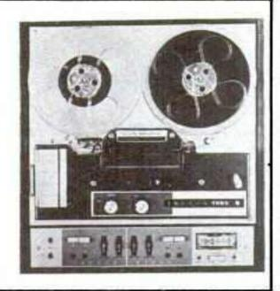
Tape speeds —  $1\frac{7}{8}$ ,  $3\frac{3}{4}$  and  $7\frac{1}{2}$  ips. Heads three. Motors — three. Record — 4-track mono and 4-track stereo. Playback — 2- and 4-track mono and 4-track stereo. Frequency response — 30-20,000 cps. Indicators — 2 meters. Weight - 40 lb. Other features - deck, with recording preamps only; 2 microphone and 2 radio-phono inputs; 2 preamp and 2 stereo headphone monitoring outputs; sound-on-sound; and built-in tape splicer. Price — \$399.50.
