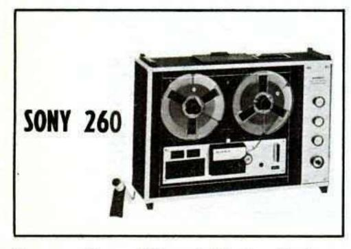
Tape speeds — 3¾ and 7½ ips. Heads — two. Motors — one. Record — 4-track mono and 4-track stereo. Playback — 4-track mono and 4-track stereo. Frequency response — 50-15,000 cps. Indicators — 2 meters. Weight — 31¾ lb. Other features — 2 microphone and 2 radio-phono inputs; 2 external speaker outputs. Built-in speakers. Price — less than \$239.50.
