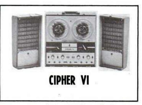
Tape speeds —  $3\frac{3}{4}$  and  $7\frac{1}{2}$  ips. Heads — two. Motors — one. Record — 4-track mono and 4track stereo. Playback — 4-track mono and 4-track stereo. Frequency response — 60-14,000 cps. Indicators — 2 meters. Weight — 38 lb. Other features — self-contained carrying case; 2 microphone and 2 radio-phono inputs; 2 preamp, 2 speaker outputs and stereo headphone; speakers in wing carrying case covers. Price **— \$239.95**.
