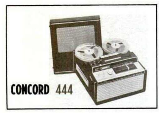
Tape speeds — 1%, 3% and 7½ ips. Heads — two. Motors — one. Record — 4-track mono and 4-track stereo. Playback — 4-track mono and 4-track stereo. Frequency response — 50-15,000 cps. Indicators — 2 neon lights. Weight — 30 lb. Other features — self-contained carrying case; 2 microphone and 2 radio-phono inputs; 2 preamp and 2 external speaker outputs; sound-with-sound; track transfer; 1 speaker built into machine and 1 speaker in case lid. Price — \$199.95.
