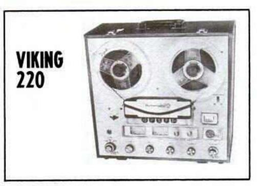
Tape speeds — 3¾ and 7½ ips. Heads — four. Motors — three. Record — 4-track mono and 4-track stereo. Playback — 4-track mono and 4-track stereo. Frequency response — 20-25,000 cps. Indicators — 2 meters. Weight — 45 lb. Other features — 2 microphone and 2 radio-phono inputs; 2 preamp, 2 external speaker, and headphone outputs; automatic reverse playback; remote control; sound-withsound; automatic shutoff. Price — \$860.
