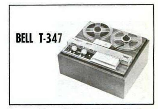
Tape speeds — 3¾ and 7½ ips. Heads — three. Motors — htree. Record — 4-track mono and 4-track stereo. Playback — 4-track mono and 4-track stereo. Frequency response — 40-16,000 cps. Meters — 2 VU. Weight — 35 lb. Other features — deck, with record and playback preamplifiers; 2 microphone and 2 radio-phono inputs; 2 preamplifier, and head-phone outputs; sound-on-sound; echo effects; electrical braking. Price — \$319.95.
