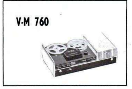
Tape speeds — 1% and 3% ips. Heads — one. Motors — one. Record — 2-track mono. Playback — 2-track mono. Frequency response — 200-6000 cps. Indicator — meter. Weight — 5 lb. Other features — powered by 10-volt nickel-cadmium battery; rechargeable; microphone and radio-phono inputs; external speaker (or earphone) output; built-in speaker. Price — \$129.95.
