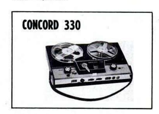
Tape speeds — 1% and 3% ips. Heads — two. Motors — one. Record — 2-track mono. Playback — 2-track mono. Frequency response — 50-10,000 cps. Indicator — meter. Weight — 6 lb. Other features — powered by 6 D-cell batteries or AC adapter; remote control microphone input; external speaker output; voice actuated recording; slide projector sync; manual tape speed control for movies. Price — \$179.95. Model 320, without slide projector sync, but with built-in AC adapter, \$129.95.
