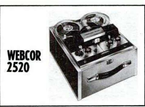
Tape speeds — 33/4 and 71/2 ips. Heads one. Motors — one. Record — 4-track mono and 4-track stereo. Playback — 4-track mono and 4-track stereo. Frequency response -50-15,000 cps. Indicator — electric eye. Weight - 27 lb. Other features - self-contained carrying case; 2 microphone inputs; 2 external speaker outputs; 2 built-in speakers. Price -\$199.95.
