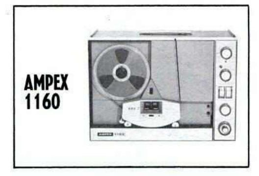
Tape speeds — 1%, 3% and 7½ ips. Heads — three. Motors — one. Record — 4-track mono and 4-track stereo. Playback — 2 and 4-track mono and 4-track stereo. Frequency response — 50-15,000 cps. Indicators — 2 meters. Weight — 38 lb. Other features — self-contained carrying case; 2 microphone and 2 radio-phono inputs; 2 speaker, accessory slide projector sync, headphone outputs; auto-
