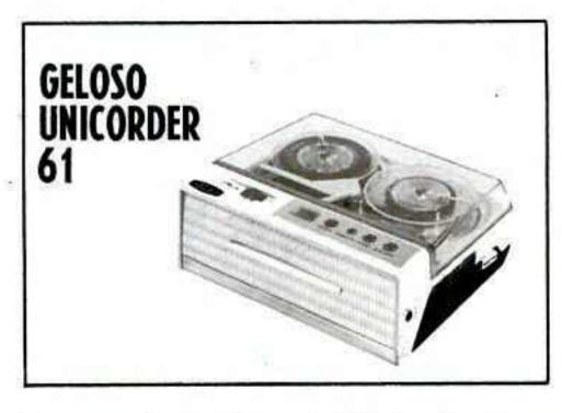
Tape speeds — 1% and 3% ips. Heads — one. Motors — one. Record — 2-track mono. Playback — 2-track mono. Frequency response — 100-5000 cps. Indicator — electric eye. Weight — 6 lb. Other features — powered by 10 penlight batteries or AC; remote control microphone and radio-phono inputs; extension speaker output; 2 built-in speakers; and strobe disc for manually controlled sync with 8mm projector. Price — \$149.95.
