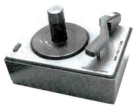
Figure 1. The RCA 45 rpm record changer.
