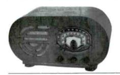
CLINTON MODEL 216 - Circa 1935-1940, this five-tube AC/DC Superhet covers standard broadcast and one shortwave band. A small brass label has the name "Clinton," and schematics of Models 149, 215 and 216 are located on the bottom of the wood cabinet. The label says Plant "A" Chicago, U.S.A. The circuit is fairly modern except that there is no automatic volume control and the "volume" control is actually RF gain. (Jay Kinnard - Austin, TX)
