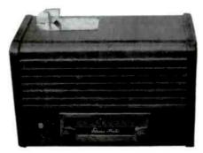
COIN-OPERATED RADIO - This is the General Electric Model YRB-12-4 AM receiver manufactured for Radio Matic of America, Inc. of Indianapolis, Indiana. The radio operates for one hour of intermittent or continuous reception for a quarter. (Tim Rall - Sharonville, OH)
