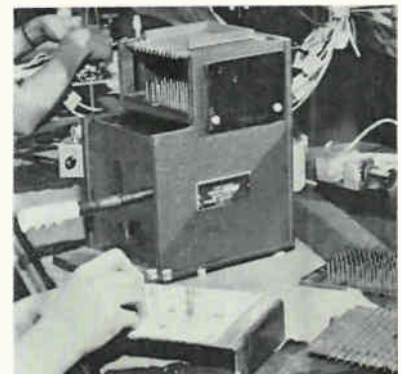
Components are placed in base plate
