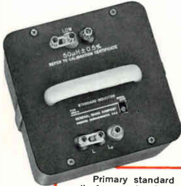
Type 1482 Standard Inductors 17 models from 50 \mu h to 10 h in 1-2-5 sequence.
