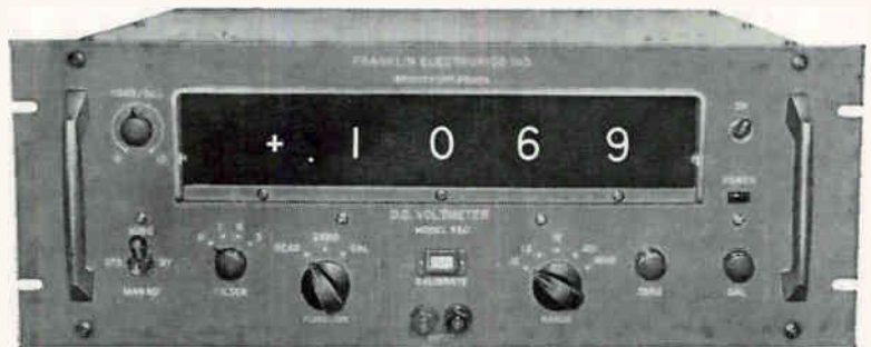
Franklin Model 550 Digital Voltmeter; \pm 0.0001 to \pm 1200 V dc; \pm 1 count accuracy; effectively infinite input impedance; automatic polarity indication; all-electronic, modular, plug-in construction.
