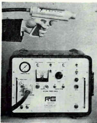
FIG. 7—Flash X-ray unit radiographs 1-in. aluminum in 0.3 \mu sec
