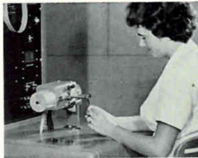
Machine is used to weld modules
