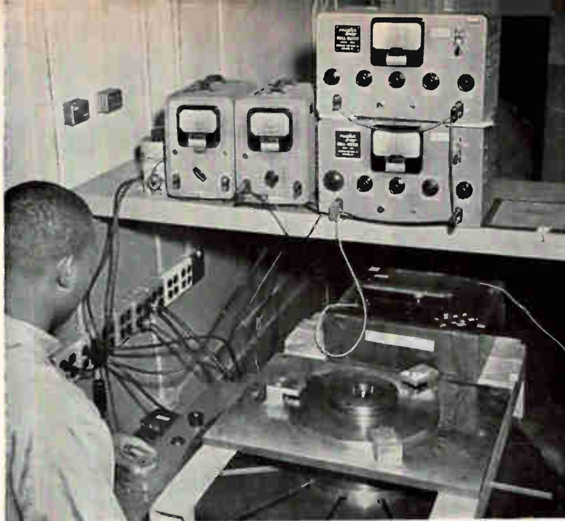
Checking the accuracy of a solid-state resolver on a two-second-accuracy index stand
