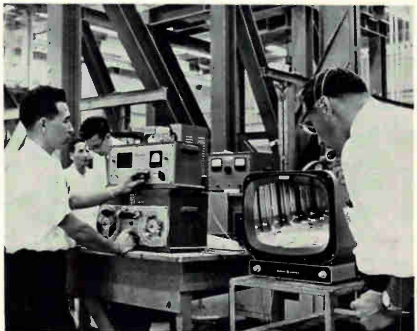
Torture tests on North American Aviation's B-70 are viewed from a safe distance by closed-circuit tv, while taped observations are recorded
