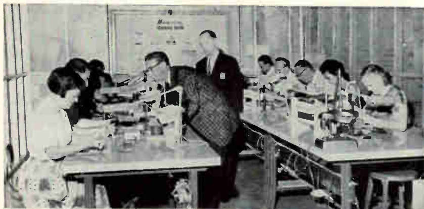
Twelve employees learn correct wiring and soldering techniques. Inexperienced operators receive 40 hours of instruction, experienced operators receive 19 hours
