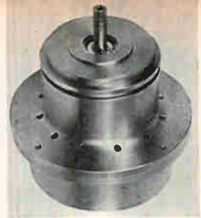
Brushless d-c motor incorporates Hall-effect commutator. Holes in this prototype permit checking of individual Hall crystals
