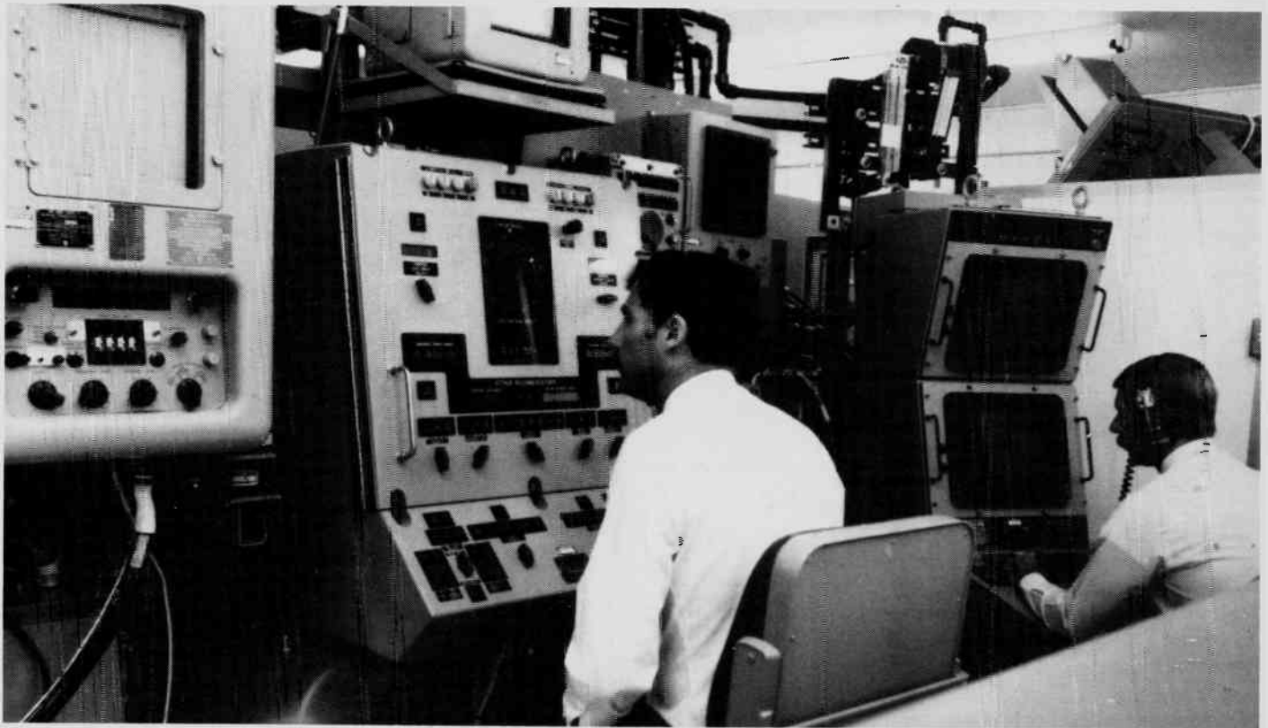
Naval training simulators such as the one above, provide crews with actual situations for using weapon systems, reducing the cost of training on actual equipment.
