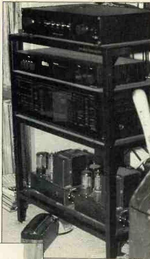
Right: The heart of the system; Croft valve pre-amplifier, Creek tuner, Nakamichi cassette deck and Leak power amplifiers below.
