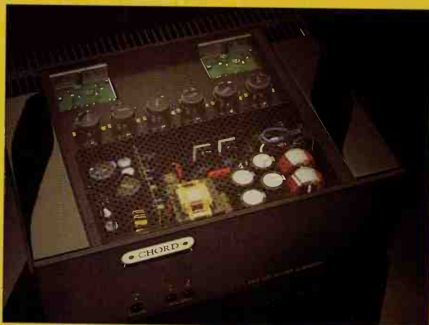
The unusual switch mode power supply with its small mains transformer and toroidal chokes (at right) can be seen at the front of the amplifier.
