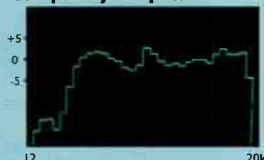
A wide bass peak centred on 100Hz should give strong bass output.
