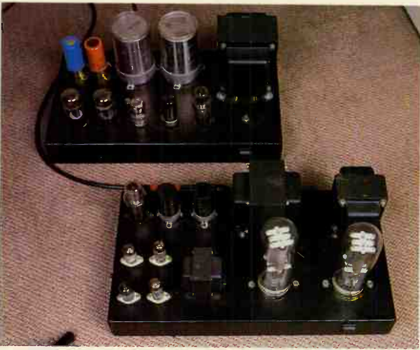
The monoblock 845 amplifier with its independent power supply (at rear) capable of 45 watts.
