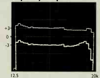
Fig 2 - The Roksan Chorus Black has a frequency response and tonal balance much like that of the K9, especially when loaded with 200pF input capacitance (lower trace). The upper trace is with signal lead capacitance only (150pF).
