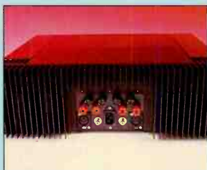
Compact dimensions restricts space for the terminals on the rear panel
