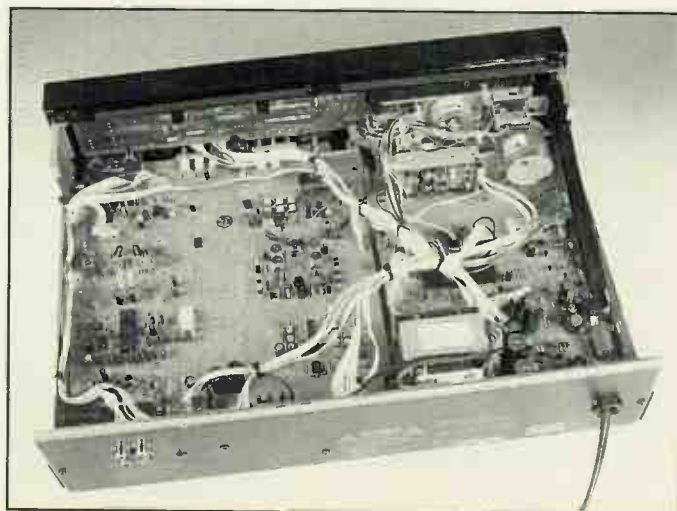
► The DR-2 three head deck with Nakamichi's own dual capstan mechanism and independent heads.
