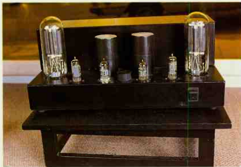
An unusual stereo power amplifier using 211s in single-ended configuration.
