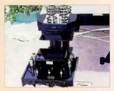
Weird, but looking wonderful: Kora valve amplification from France, which uses the rare and peculiar Russian 6C33C triode valve, reputedly for "trawler" transmitters.
