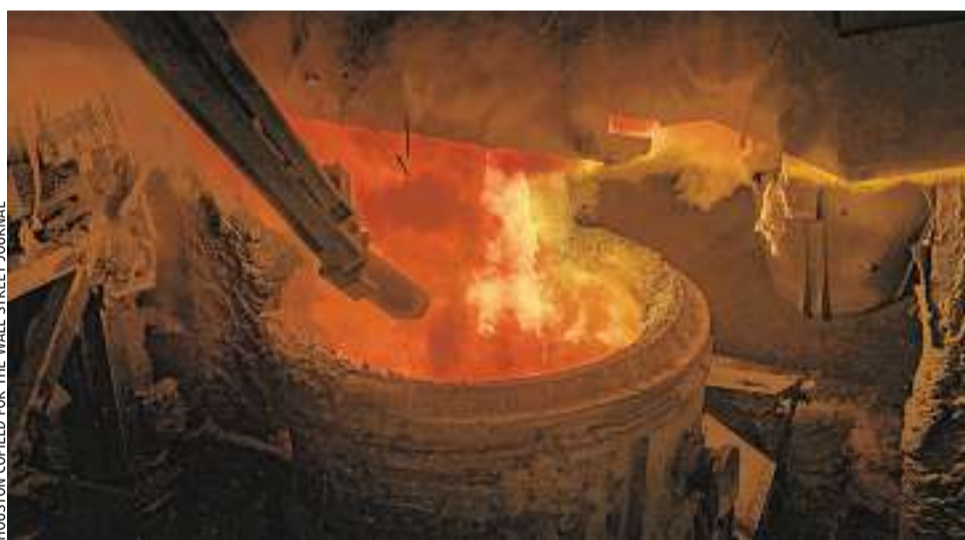
Molten metal is poured into a crucible before being formed into steel bars. Production is rising.
