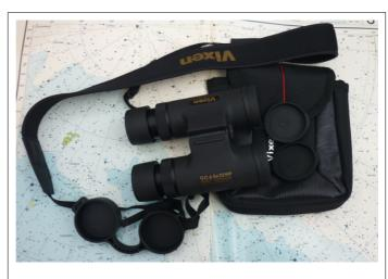
are an excellent fit, and do not come off accidentally; they are fitted with tabs to aid uncapping. They can be completely removed from the binocular if you don't like dangling covers when you are observing. The eyepieces have a tetherable (right hand side, with a split loop for the left hand strap) rainguard-type cover that fits securely. It does not to restrict the interpupillary distance when it is in place.
