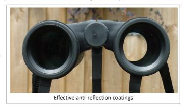
ribbed at the objective end, suggesting that control of stray light should be good. There are no cutoffs in the light path, suggesting that the prisms are adequately sized. The prisms are specified as being BK7 (lower dispersion than BaK-4) and "special elements of less absorption of light" that are fully multicoated (FMC) on their transmissive surfaces and to have phase correction coatings (PC) and Vixen's proprietary super high-reflectivity coatings (SHRC) on the reflective surfaces.
