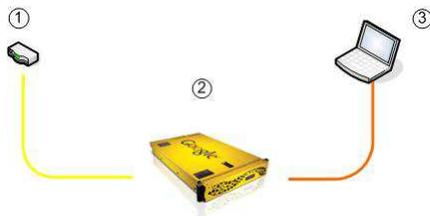
1. Network router connected to search appliance by the yellow Ethernet cable, which is the longer of the two cables supplied with the search appliance.
