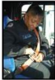
Installing the E-Clip. Lowers belt angle and lessens "neck rub".
