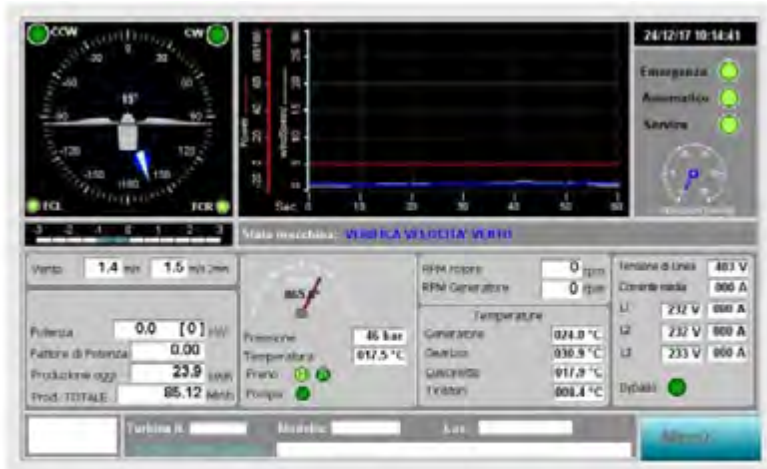
The controls for this wind turbine are located in Italy. According to additional screenshots found on the turbine manufacturer's website (name deleted for privacy), all aspects of the turbine, i.e., start, stop, reset, and system parameters, can be controlled using this software.
