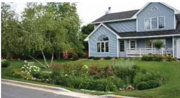
Rain gardens filter stormwater runoff before it soaks into the ground.
