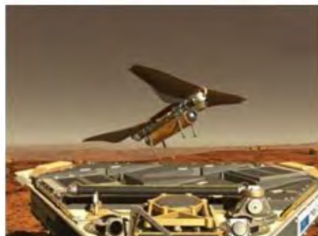
Figure 1-10: Animation of Entomopter Mission (Take off, Flight, Sample Gathering, and Return to the Lander)
