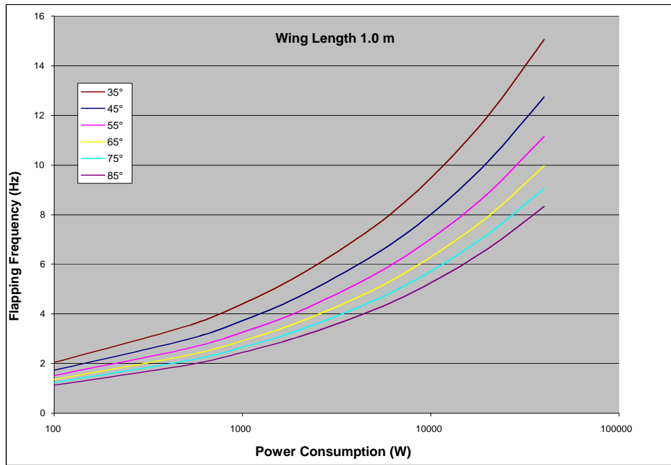
Figure B-9: Flapping Frequency vs. Power Consumption (Watts) for a Wing Length of 1.0 m
