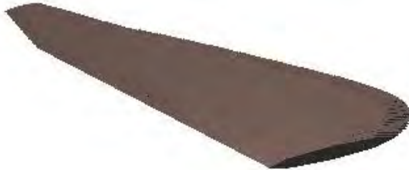
Figure 3-25: CAD Wing Section for the Hollow, Tapered Baseline Geometry--Root to Tip from Wing Top
