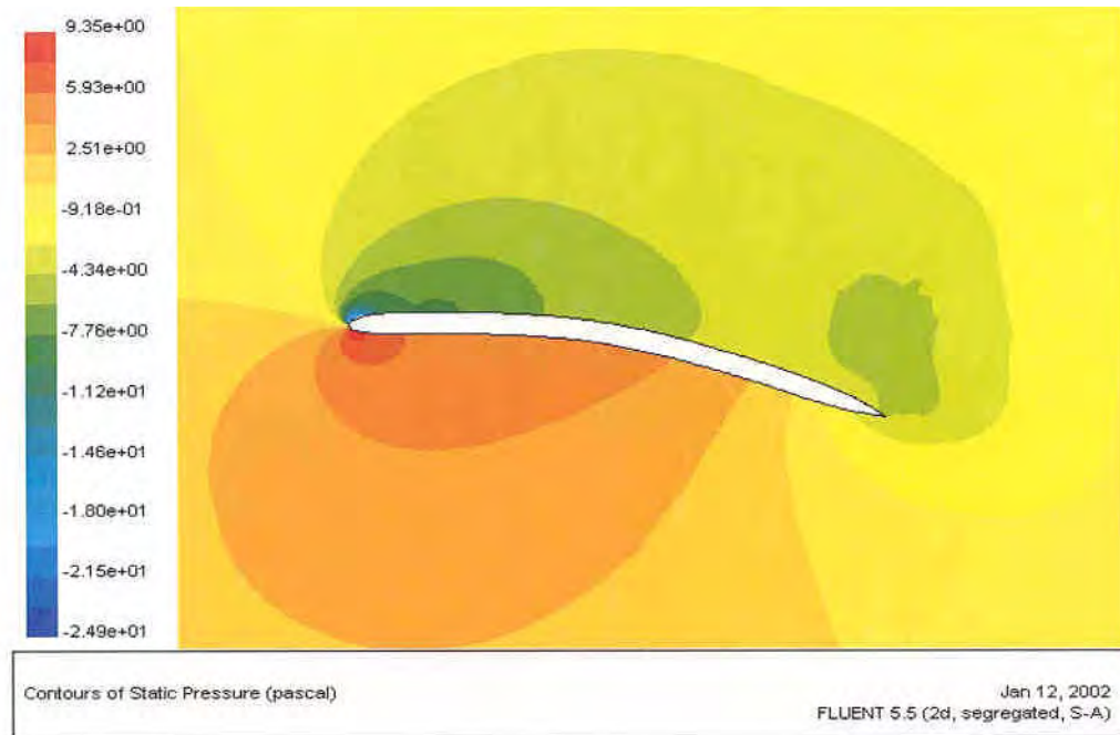
Figure 3-58: Pressure Contours for \alpha = 17.31^\circ
