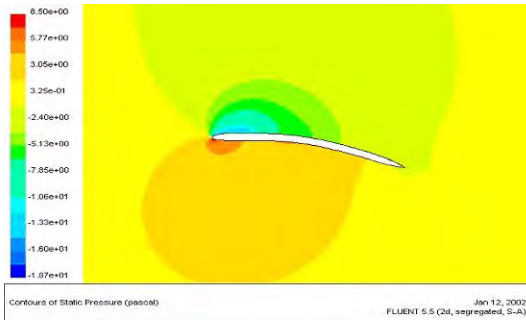
Figure 3-54: Pressure Contours for \alpha = 11.31^\circ
