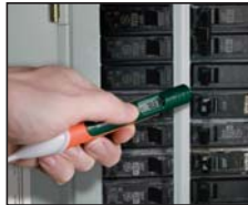
Non-contact InfraRed Temperature measurement
