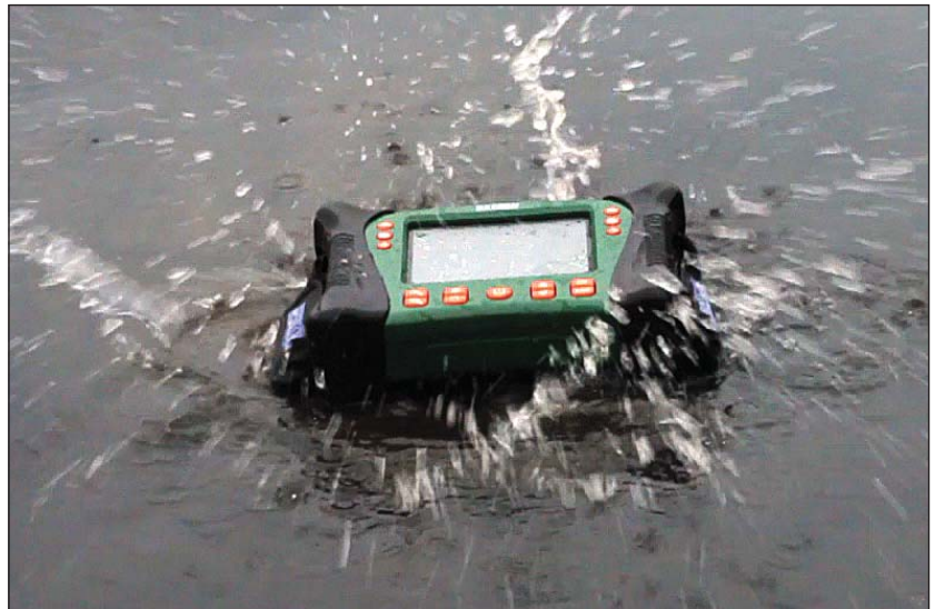
Drop proof and Waterproof housing meets IP67 standards
