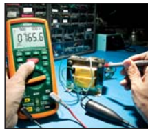
Measure the insulation resistance of transformer windings
