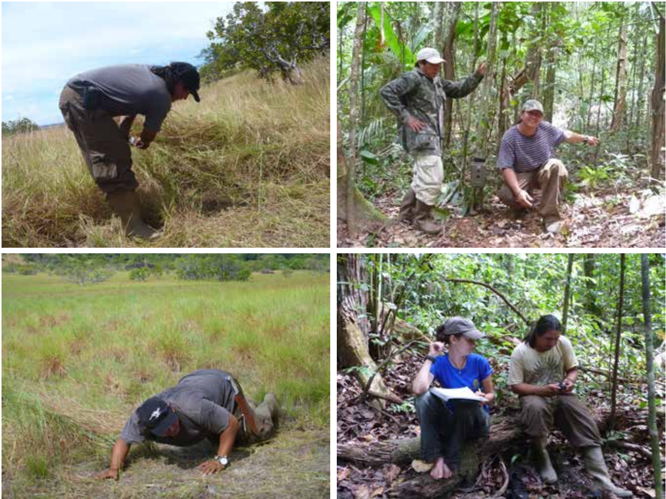
Figure 5.1 Camera trap set-up process: (clockwise) clear viewing area; attach camera; test the camera with the crawl test; and record camera station data, including GPS point and habitat information.
