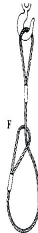
Fig. 7f. Choker Hitch One leg vertical, with slip-through loop Rated capacity is 75% of the single rope in Fig. 7a.
