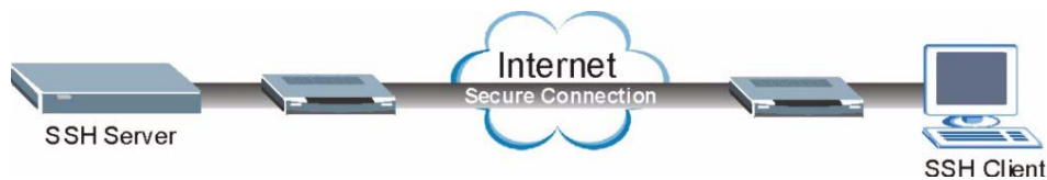
Figure 159 SSH Communication Example
