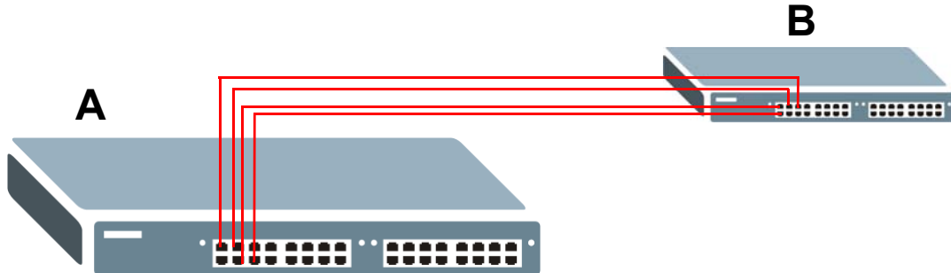
Figure 83 Trunking Example - Physical Connections
