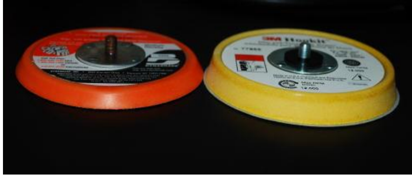
Figure 5 : Sanding discs showing variable padding thicknesses.
