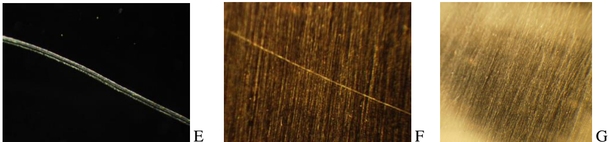
Figures E-G: Progressive removal of a large scratch by sanding.
