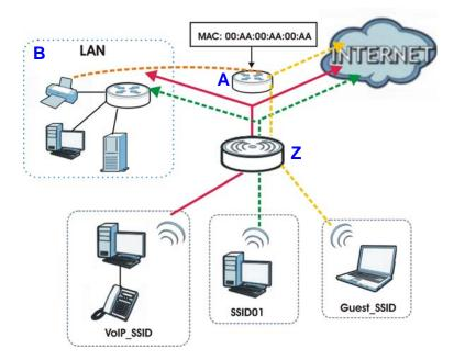
The standard network (**SSID01**) has access to all resources. The VoIP network (**VoIP\_SSID**) has access to all resources and a high QoS priority. The guest network (**Guest\_SSID**) has access to the Internet and the network printer only, and a low QoS priority.
