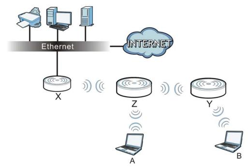
When the NWA is in Repeater mode, repeater security between the NWA and other repeater is independent of the security between the wireless clients and the AP or repeater. If you do not enable repeater security, traffic between APs is not encrypted. When repeater security is enabled, both APs and repeaters must use the same pre-shared key. See Section 6.6 on page 73 for more details.
