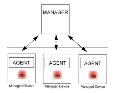
An SNMP managed network consists of two main types of component: agents and a manager.
