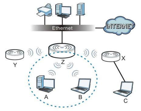
On the NWA in Root AP mode, you can have multiple SSIDs active for regular wireless connections and one SSID for the connection with a repeater (repeater SSID). Wireless clients can use either SSID to associate with the NWA in Root AP mode. A repeater must use the repeater SSID to connect to the NWA in Root AP mode.
