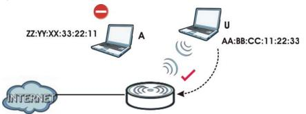
In the figure above, wireless client  $\mathbf{U}$  is able to connect to the Internet because its MAC address is in the allowed association list specified in the NWA. The MAC address of client A is either denied association or is not in the list of allowed wireless clients specified in the NWA.
