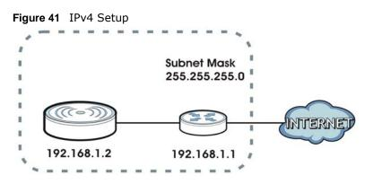
The figure above illustrates one possible setup of your NWA. The gateway IPv4 address is 192.168.1.1 and the IPv4 address of the NWA is 192.168.1.2 (default). The gateway and the device must belong in the same subnet mask to be able to communicate with each other.
