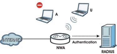
In the figure above, wireless clients **A** and **B** are trying to access the Internet via the NWA. The NWA in turn queries the RADIUS server if the identity of clients **A** and **U** are allowed access to the Internet. In this scenario, only client **U**'s identity is verified by the RADIUS server and allowed access to the Internet.
