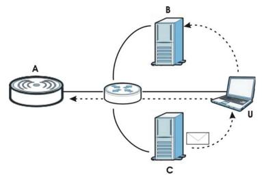
The figure above illustrates three ways to access logs. The user (U) can access logs directly from the NWA (A) via the Web configurator. Logs can also be located in an external log server (B). An email server (C) can also send harvested logs to the user's email account.
