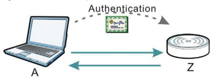
In the figure above, the NWA (Z) checks the identity of the notebook (A) using a certificate before granting access to the network.
