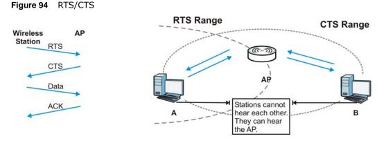
When station **A** sends data to the AP, it might not know that the station **B** is already using the channel. If these two stations send data at the same time, collisions may occur when both sets of data arrive at the AP at the same time, resulting in a loss of messages for both stations.
