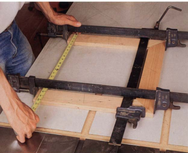
Three clamps pull the miters together and prevent the pieces from slipping when the leg-and-apron units are glued up.
