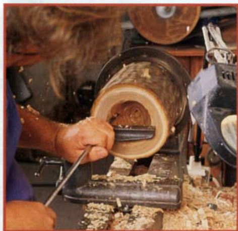
To hollow out a birdhouse, the author first drills a 1/2-in.-dia. hole for a hook tool, so he can work from the center toward the edge to avoid cutting into the endgrain.
