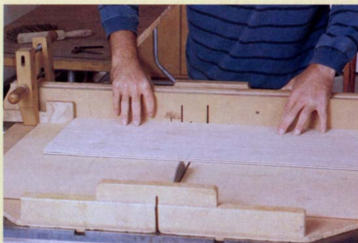
Voorhees crosscuts the vertical side panels for his box-drawer construction from a single piece of plywood, after ripping the grooves that will receive the horizontal drawer dividers. Ripping the grooves first and then crosscutting the panel, ensures that the grooves on opposite sides of the case will matchup perfectly.
