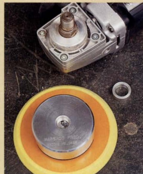
The Marshco attachment on a body grinder is a cost-effective way to access random-orbit sanding. The attachment's backing pad uses PSA-type discs.
