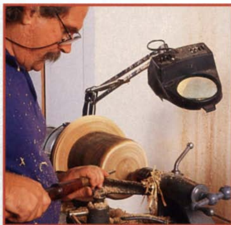
Turning the bottom of the birdhouse to a uniform thickness helps prevent checking. The blank is mounted on a jam chuck and supported between centers.
