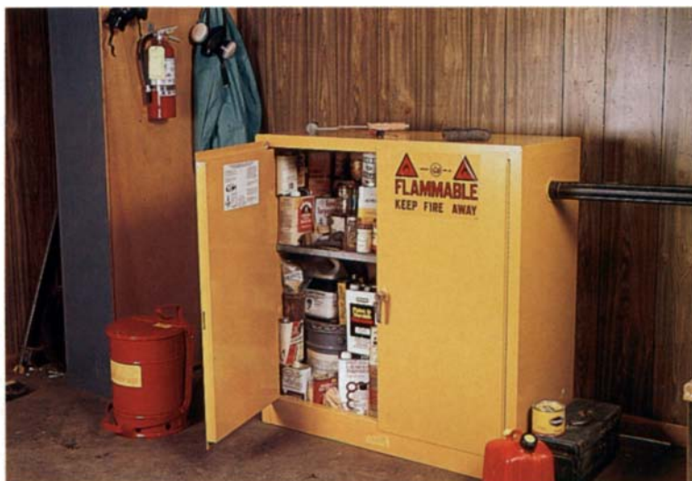
Flammable chemicals should be stored in a steel cabinet that is vented to the outside. A lidded, metal bucket (at left above) provides temporary safe storage for solvent-laden rags.
