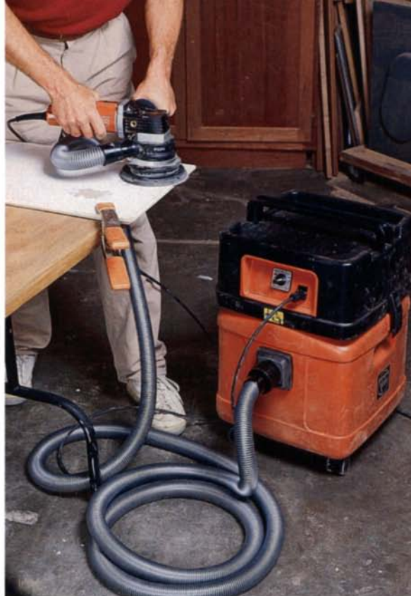
The dust collection system for the Fein MSf 636 includes the optional 920 13 shop vacuum. By plugging the sander into the vacuum, the vac is turned on and off automatically with the sander.
