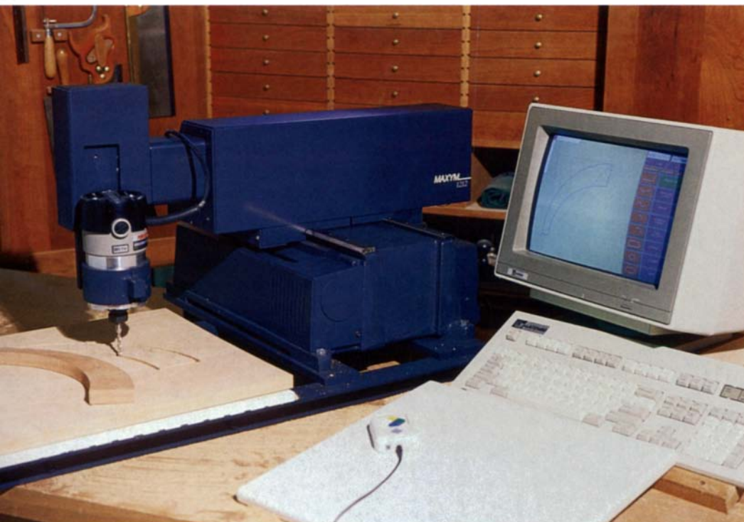
The Maxym robot is a mechanized-milling machine run by a personal computer. Shapes can be programmed easily and quickly by drawing them on a digitizing tablet (shown in front of the computer). Then the machine employs a regular router and spiral end mill to perform the desired task. Here, the Maxym robot has been programmed to cut out a curved chair part as an experiment for Thos. Moser Cabinetmakers.
