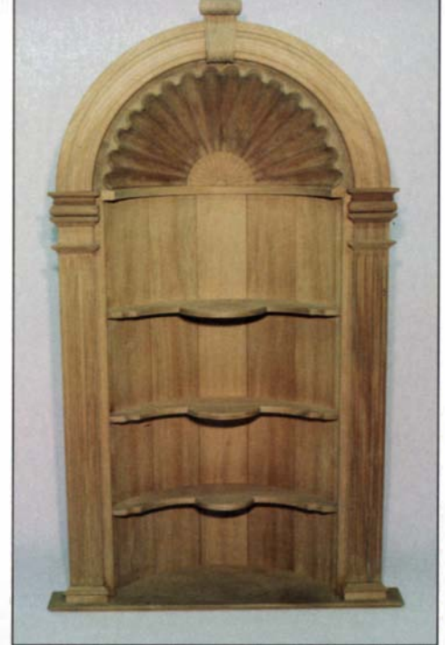
A clear-finished shell glued up from compound, angled segments has a more consistent color across the interior of the shell than the checkerboard pattern of endgrain and long grain found in the typical layered shell.
