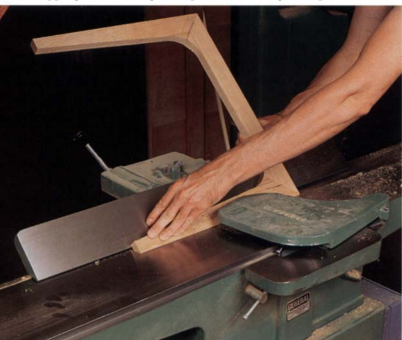
Mitering the edges of the legs on the jointer is easier and provides better results than doing them on the tablesaw.
