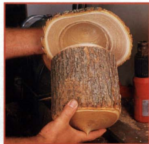
A lip turned on the top edge of the body fits into a recess turned into the underside of the roof. Beeswax is used to seal and protect all exterior surfaces.
