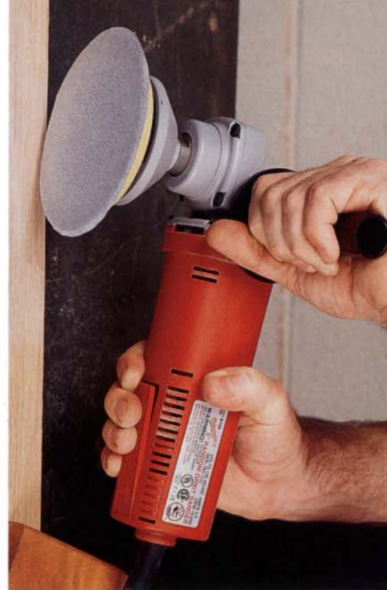
The switch on the Milwaukee 6125 is an easy-to-press flap on the underside of the motor housing. Hanson found this switch to be the safest and most comfortable to use.
