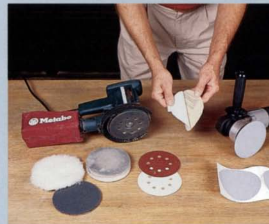
The two methods for attaching sanding discs to random-orbit sanders are the hook-and-loop system, left, and the pressure-sensitive-adhesive system, right.
