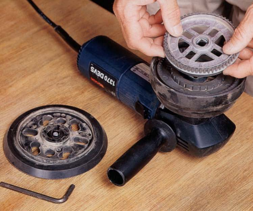
The convertible drive system on the Bosch 1370DEVS machine, left, allows the sanding aggressiveness to be adjusted. Beneath the backing pad is a reversible drive ring that can be installed one way for direct drive (heavy sanding) and then flipped over, in about one minute, for “slip drive” (sensitive sanding).
