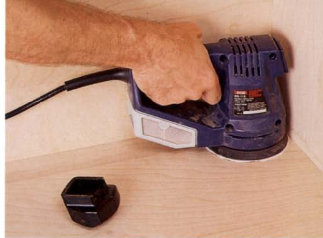
The Ryobi RS-115 easily sands into corners once its detachable front handle has been removed (above). The plastic-screen dust container nestled below the rear handle slides off for emptying.
