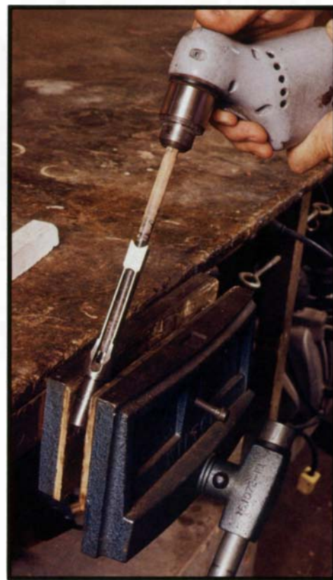
Polishing a chisel's interior: After rubbing the chucked dowel with white rouge, the author inserts it into the hollow chisel. The wooden dowel is soft enough that there is no danger of damaging the chisel while the rouge mildly abrades and polishes its interior passageways.
