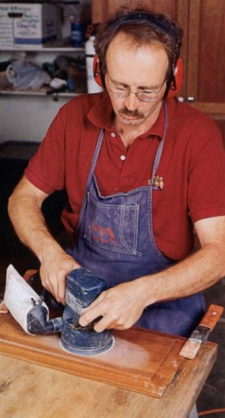
While sanding a lacquer finish with the Bosch 3283DVS, the author strives to keep the machine absolutely flat on the cherry panel.
