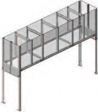
Frame Supported Exhaust Duct
