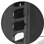
Fingers align with RMU on rack
