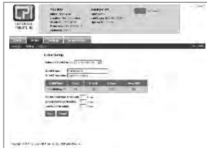
Outlet Set-Up - Ability to set alarms for upper and lower current thresholds for each outlet
