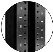
Rack-Mount Unit (U) marks simplify equipment installation
