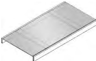
Tray rests on cross members between stringers.
