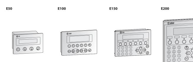
The **E50** is a key-oriented HMI unit with four function keys and an LCD display with two rows and 16 characters each. It can display up to 50 text blocks, which can be paged with the function keys. Values can be edited directly with the unit's keyboard. The RS232C and RS422 ports are both integrated in a 25-pin connector.
