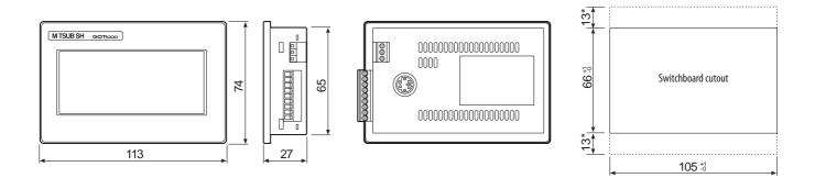
\* A space of at least 13 mm at the long side of the GOT is required to allow for the attachment of mounting fixtures.
