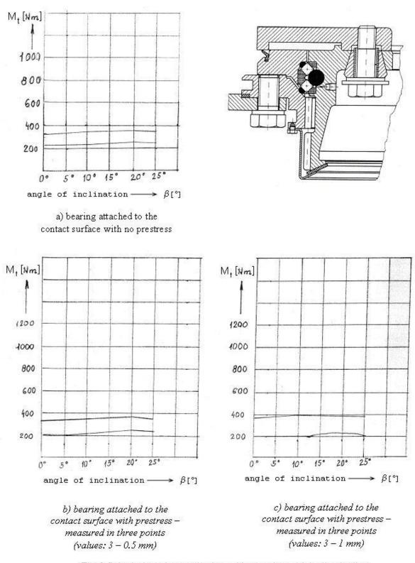
Expression of  $M_t$  torque resistance depending on  $\beta$  inclination angle and prestress for spherical T-72 turnet turning mechanism with a double-row roller bearing (appropriate):
