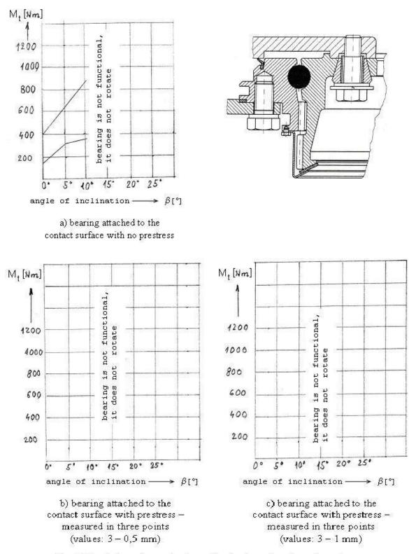
Expression of Mt torque resistance depending on  $\beta$  inclination angle and prestress for the spherical turret swivel:
