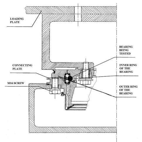
Fig. 5 Testing device for the T–72 M2 bearing
