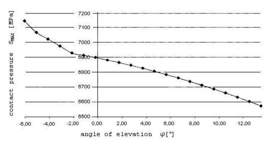
Fig. 4 Dependence of the contact pressure on the angle of elevation of the cannon
