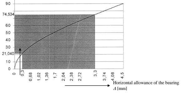
Fig. 3  $\beta$  contact angle dependence on  $\Delta$  horizontal allowance of the T–72 tank bearing
