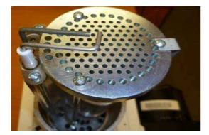
**Step 5:** Refit the electrode assembly and ensure the connections are secure to prevent incorrect sparking of the spark electrode.
