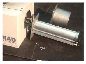
**Step 1.b:** The burner head assembly can be disconnected by separating the connectors of the ignition lead assembly and removing the pressure switch silicon tube.
