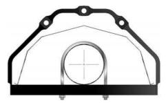
Type 'F' is a fixed reflector support bracket and are fixed to the reflector via set screws.
