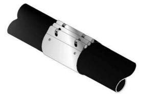
Slide the coupler over the tube ensuring that the rivet stop has butted up to the tube ends. Using an Allen wrench, tighten the pins.
