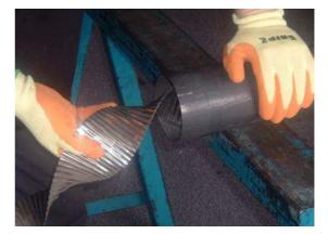
**Step 5:** The turbulators should be cleaned with a soft brush.
