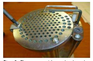
**Step 2:** The pepper pot burner head can be replaced ensuring the 5 holes on the outer ring are aligned alongside the probes.
