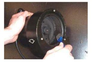
**Step 6:** Remove any dust from fan scroll and from around the motor.
