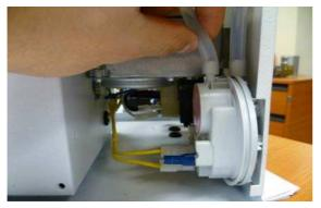
**Step 4:** Remove the 4 screws holding the burner head onto the burner assembly.
