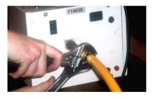
**Step 4:** If ducted air is connected, loosen hose clamp and remove the flexible hose from the burner.
