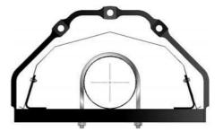
Type 'B' is a sliding reflector suspension bracket and NOT fastened to the reflector. They are fixed at regular intervals down the length of the tube.
