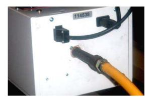
**Step 3:** Detach the gas supply as shown below, taking care to support the burner connection.
