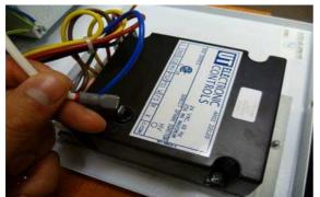
**Step 4:** Remove the two screws attaching the controller to the burner door and remove.
