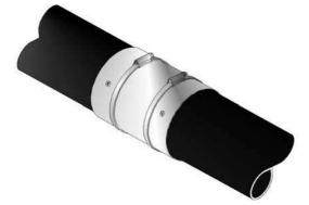
Slide the coupler over the tube ensuring that the tube stop has butted up to the tube ends. Using a 5/16" drive or flat blade screwdriver, tighten the bolts.
