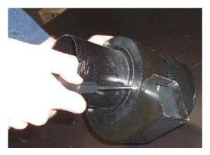
**Step 5:** Inspect the impeller and remove any dust with a soft brush.
